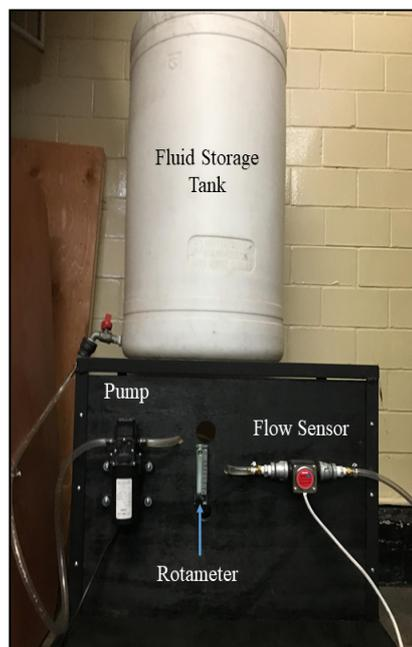
Figure 5. Flow control module prototype.
