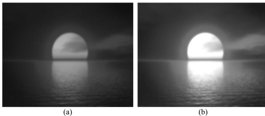
Fig. 4. Two image of the same scene captured at different exposure times: (a) 10 milliseconds and (b) 20 milliseconds.
