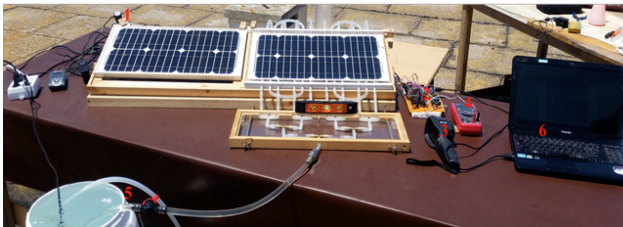
Fig. 1. PVT system. (1) Solarimeter-SL 200; (2) Control and data acquisition board; (3) Thermal camera; (4) Thermocouple; (5) Adjustable flow rate water pumping system; (6) Data recording (Computer).
