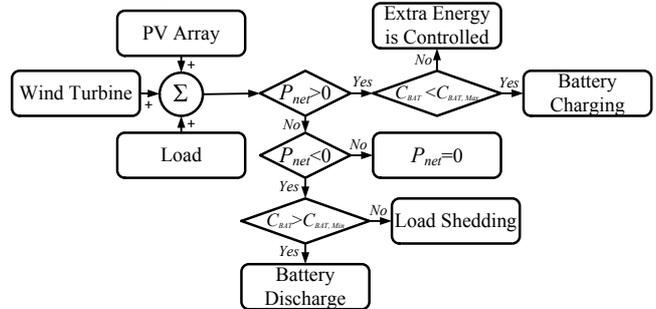
Fig. 5. The block diagram of the proposed hybrid energy system
