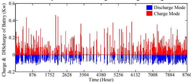
**Fig. 16.** The battery set annual charge/discharge changes for selected hybrid system
