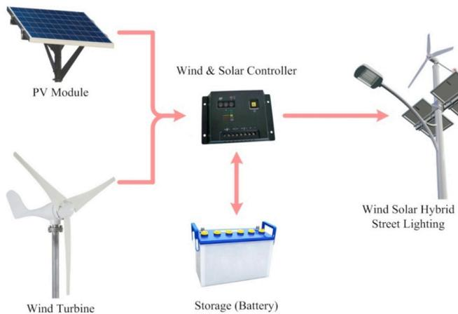
**Fig. 4.** General configuration of hybrid system for highways and street lighting
