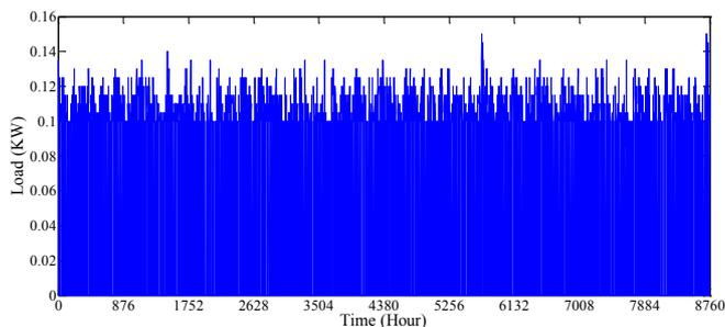
**Fig. 8.** Forecasted load profile of under study system (each light) for a year
