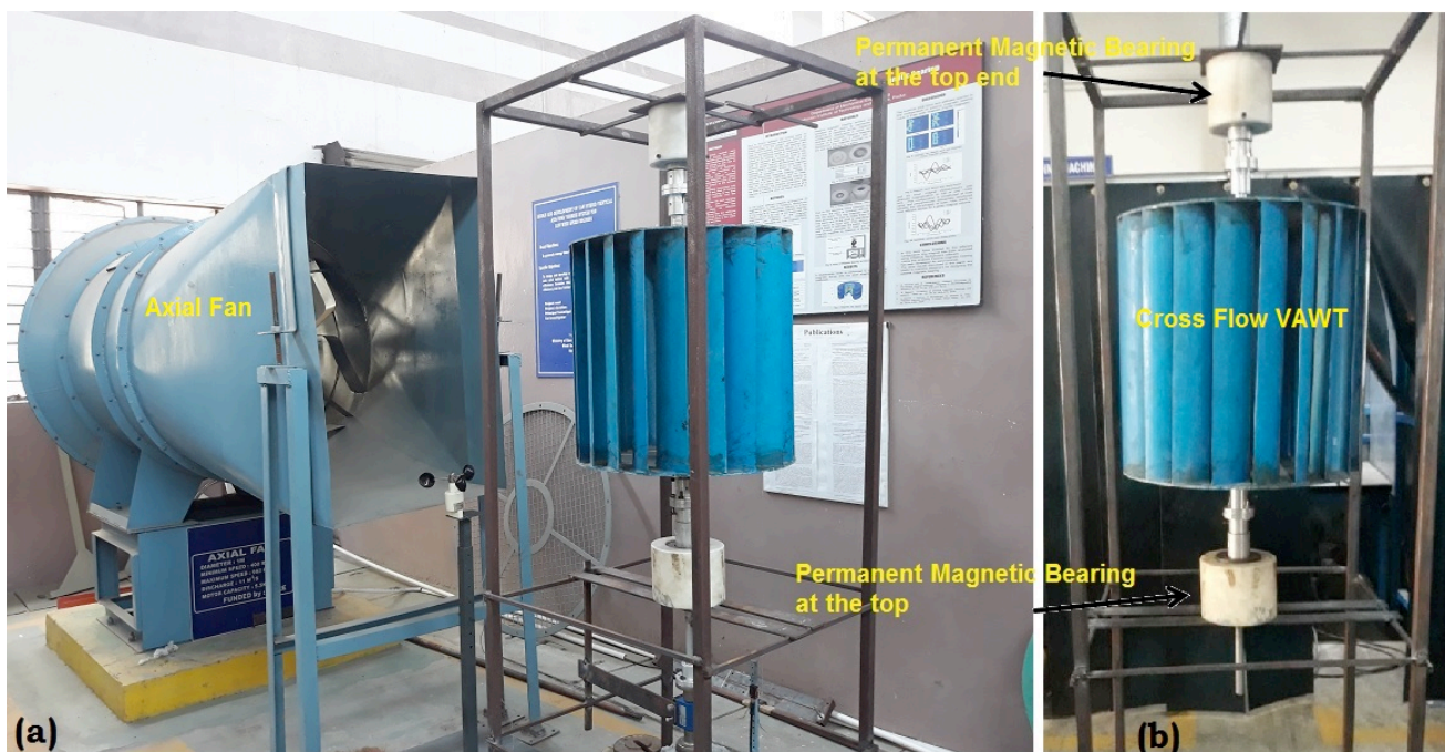
Fig.13. Experimental setup of the tested prototype PPMB with cross flow VAWT
