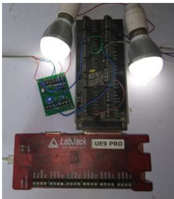
Fig. 8. PV Tracker control and load circuit.
