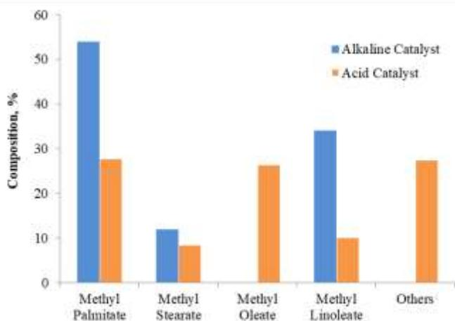
**Fig. 7.** Comparison of FAME composition of biodiesel in using alkaline and acid catalyzed extractive-transesterification.
