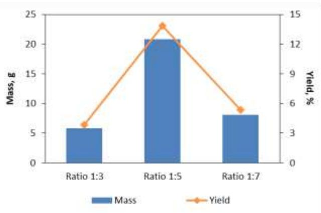
**Fig. 8.** Comparison of biodiesel mass and yield on various biomass weight-solvent volume ratios.
