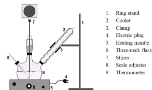
**Fig. 1.** Equipment set for extractive-transesterification [45].
