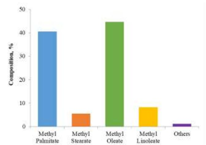
**Fig. 4.** FAME composition of biodiesel from *Arthrospira sp.* using alkaline catalyzed conventional two-step process.
