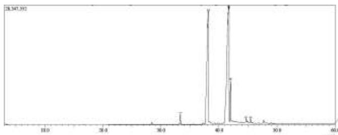
**Fig. 3.** The GC-MS result of biodiesel from *Arthrospira sp.* using alkaline catalyzed conventional two-step process.
