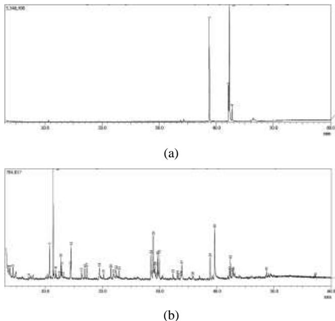
**Fig. 6.** The GC-MS result of biodiesel from *Arthrospira sp.* using: (a) alkaline (sodium hydroxide); (b) acid (sulfuric acid) catalyzed extractive-transesterification.
