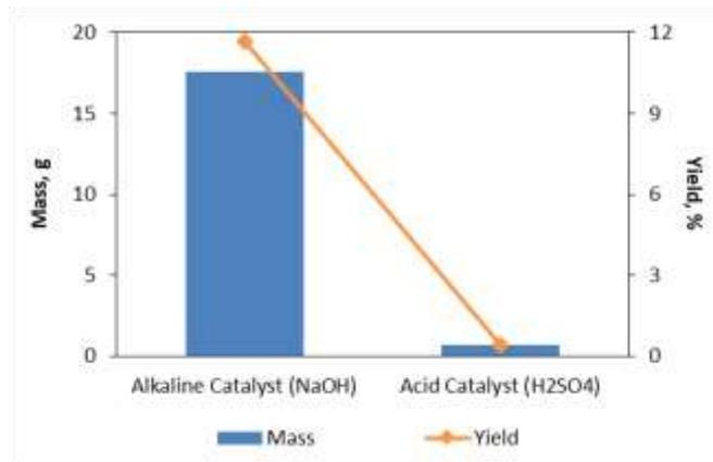
**Fig. 5.** Comparison of biodiesel mass and yield in using alkaline and acid catalyzed extractive-transesterification.
