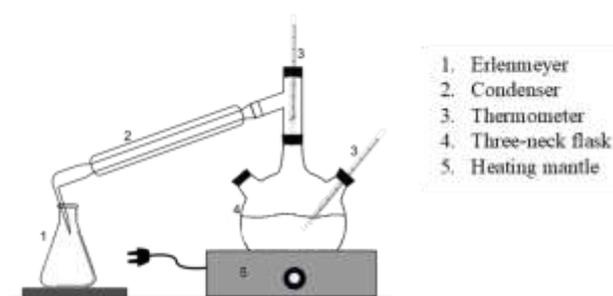
**Fig. 2.** Equipment set for washed-biodiesel purification.
