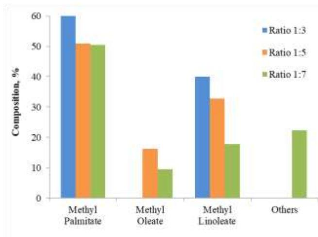
**Fig. 9.** FAME composition of biodiesel on various biomass weight-solvent volume ratios.
