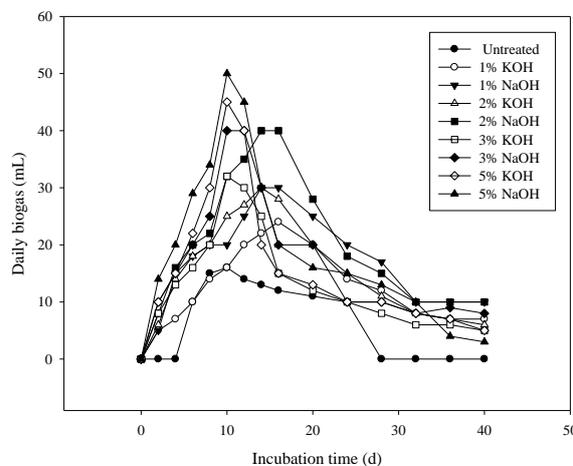
**Fig 7.** Daily volumetric biogas of 1,2,3 and 5% NaOH and KOH pretreated almond shell.
