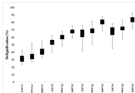
**Fig 1.** Box plot demonstration of comparative delignification for 1-5% NaOH concentrations. WT= water bath, Auto= autoclaving, MW= microwave
