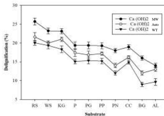
**Fig 4C:** Comparative delignification of 0.5% Ca(OH)<sub>2</sub> for microwave (MW), autoclave (Auto), and water bath (WT). P =paper, WS= wheat straw, RS=rice straw, PG=para grass, KG= kalar grass, BG=bagasse, PP=pulse peel, PN = peanut, CC=corn cob, AL=almond.
