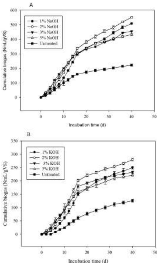
**Fig 8.** Cumulative biogas of 1,2,3 and 5% NaOH and KOH pretreated wheat straw.
