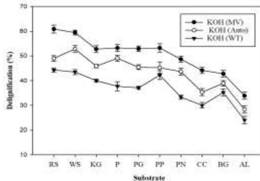
**Fig 4B:** Comparative delignification of 2% KOH for microwave (MW), autoclave (Auto), and water bath (WT). P =paper, WS= wheat straw, RS=rice straw, PG=para grass, KG= kalar grass, BG=bagasse, PP=pulse peel, PN = peanut, CC=corn cob, AL=almond.
