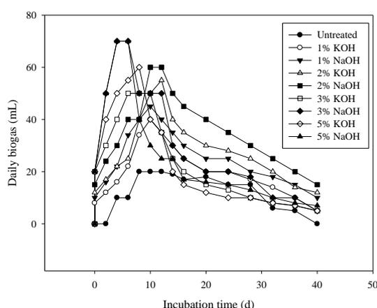
**Fig 6.** Daily volumetric biogas of 1,2,3 and 5% NaOH and KOH pretreated wheat straw.
