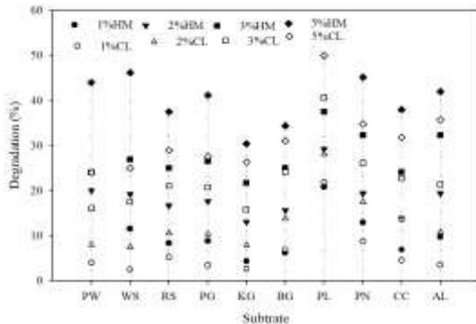
**Fig 3.** Effect of 1-5% NaOH concentrations on holocellulose degradation. HM= hemicellulose, CL=cellulose, PW =paper waste, WS= wheat straw, RS=rice straw, PG=para grass, KG= kalar grass, BG=bagasse, PP=pulse peel, PN = peanut, CC=corn cob, AL=almond.
