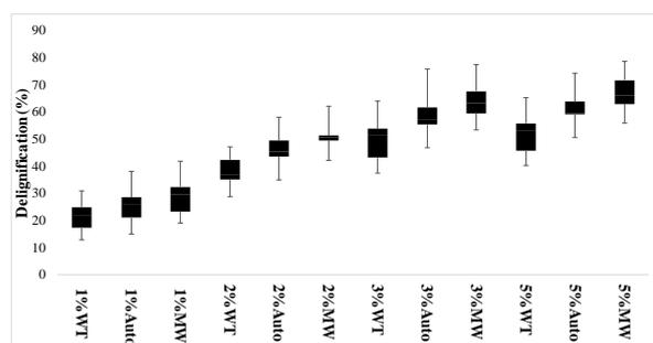
**Fig 2.** Box plot demonstration of comparative delignification for 1-5% KOH concentrations WT = water bath, Auto= autoclaving, MW= microwave
