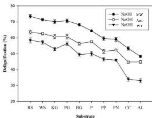
**Fig 4A:** Comparative delignification of 2% NaOH for microwave (MW), autoclave (Auto), and water bath (WT). P =paper, WS= wheat straw, RS=rice straw, PG=para grass, KG= kalar grass, BG=bagasse, PP=pulse peel, PN = peanut, CC=corn cob, AL=almond.
