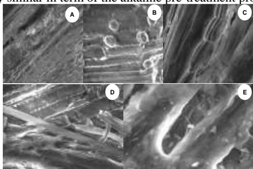
**Fig. 5.** Morphology of the wheat straw solid fraction after the pre-treatment by SEM micrographs for the untreated and pre-treated with 1-5% NaOH (A) untreated (B) 1% NaOH treated (C) 2% NaOH treated (D) 3% NaOH (E) 5% NaOH treated wheat straw with equal magnification.
