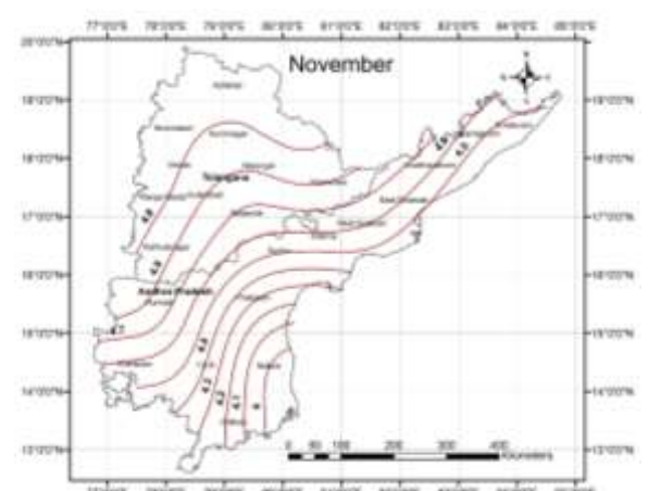
Fig. 19. Contour map of solar radiation ( \text{kW h/m}^2 \text{ day} ) for AP and TS (November).
