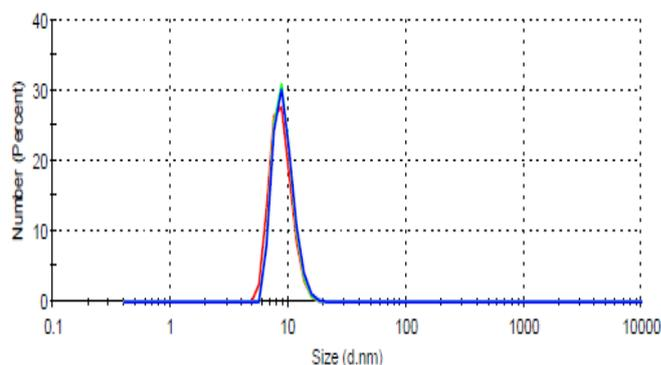
**Fig. 2.** Particle size distribution of CDs derived from rice husk
