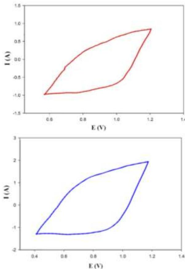
**Fig. 7.** Cyclic voltammogram of  $\text{MnO}_2/\text{CDs}$  nanocomposite electrodes with addition of (above) 75 mL and (below) 125 mL of CDs solution
