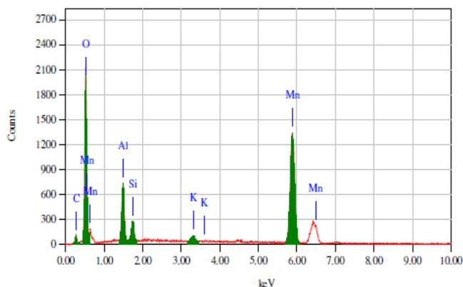
**Fig. 5.** EDXS spectrum of MnO<sub>2</sub>/CDs nanocomposite
