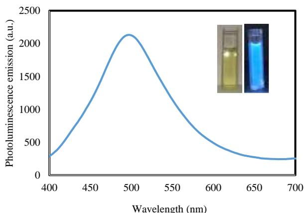
**Fig. 1.** Photoluminescence emission spectra of CDs derived from rice husks.
