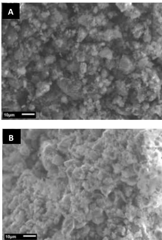
**Fig. 4.** SEM images of MnO<sub>2</sub>/CDs nanocomposite with the addition of (A) 75 mL and (B) 125 mL of CDs solution
