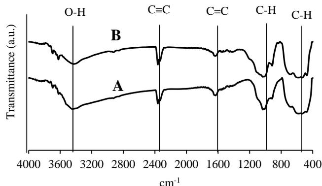
**Fig. 6.** FTIR spectra of MnO<sub>2</sub>/CDs nanocomposite
