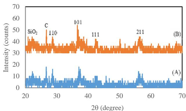
**Fig. 3.** XRD pattern of MnO<sub>2</sub>/CDs nanocomposites with the addition of (A) 75 mL and (B) 125 mL of CDs solution.
