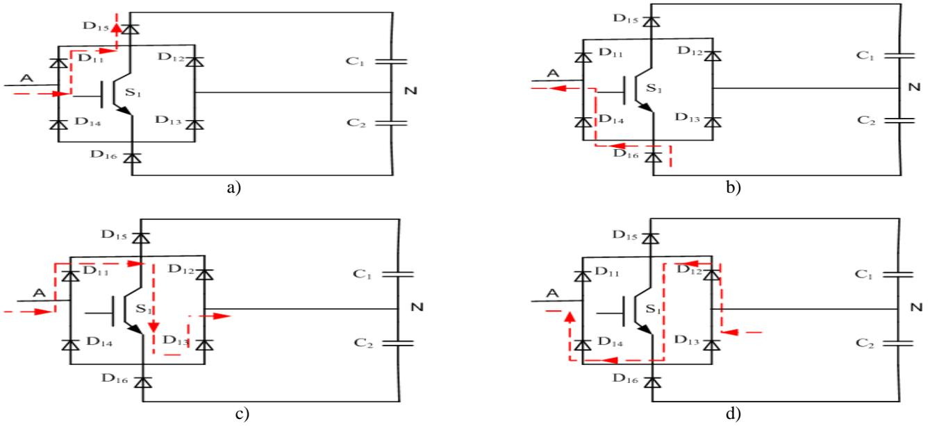
**Fig.3** Current flow in the circuit when  $S_1=0$  (Fig3a:  $I_A +ve$  & Fig3b:  $I_A -ve$ ) and  $S_1=1$  (Fig3c:  $I_A +ve$  & Fig3d:  $I_A -ve$ )
