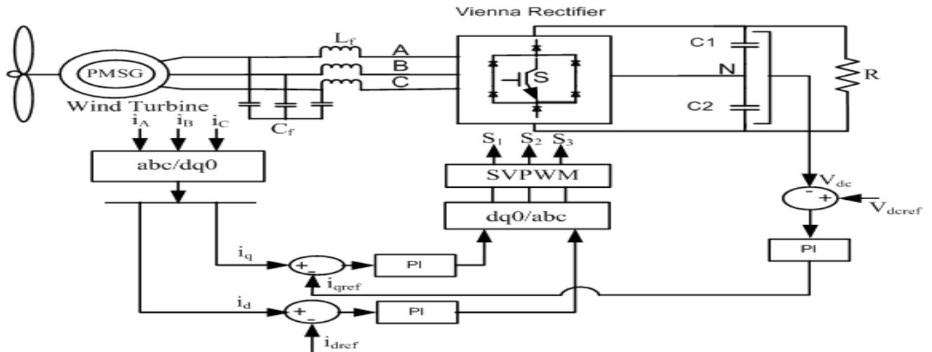
Fig.4 Proposed model of an SVPWM based three phase boost type Vienna Rectifier
