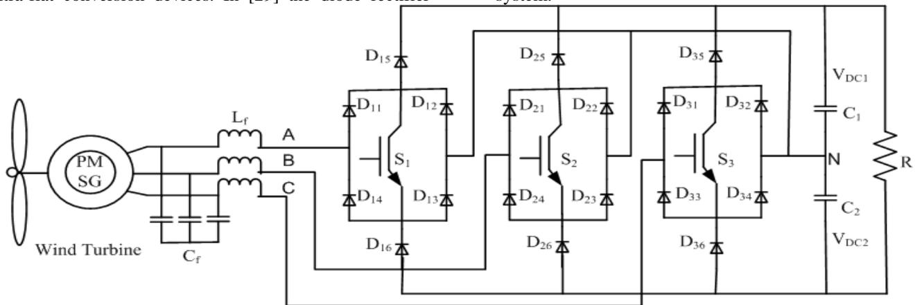
**Fig.1** Proposed circuit model of a 3- $\phi$  boost type Vienna Rectifier
