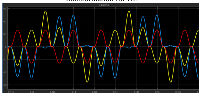
Fig. 13. M1 I_{L\alpha\beta 0} waveforms after using Clarke's transformation for L1.
