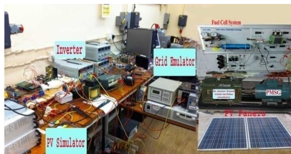
Fig. 24 Experimental hybrid controller using dSPACE platform
