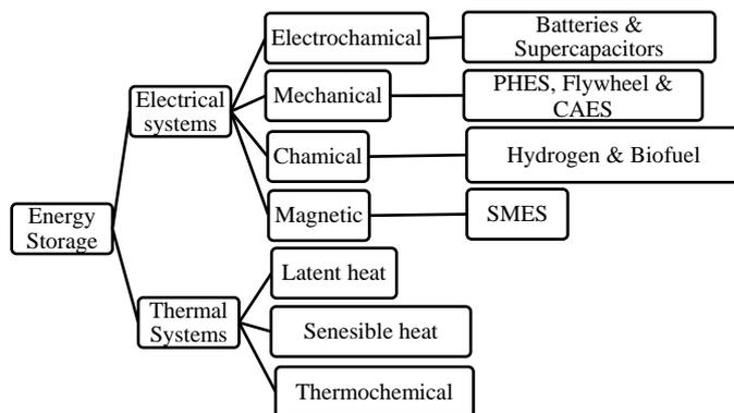
Fig. 1. Classification of energy storage technologies
