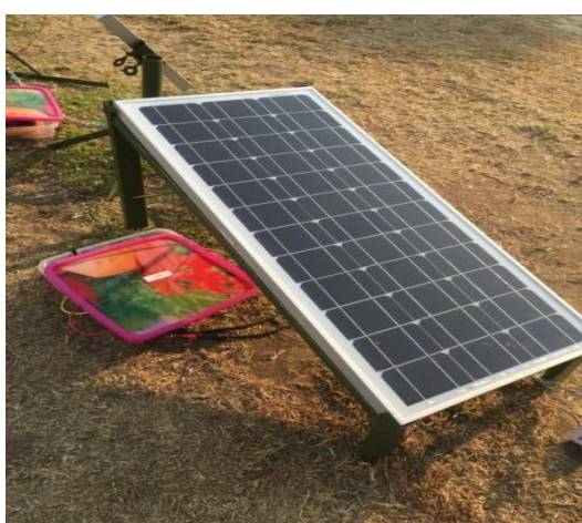
Fig. 2. Experimental setup of non-cooling system.
