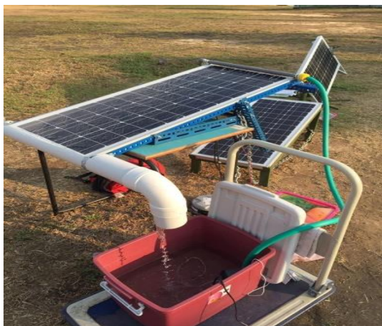
Fig. 1. Experimental setup of cooling system.
