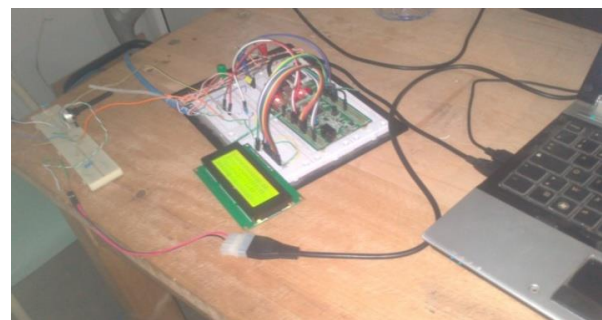
Fig. 14. Connection between LCD Display and STM32F4 Board.
