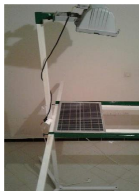
Fig 13 Support for PV panel
