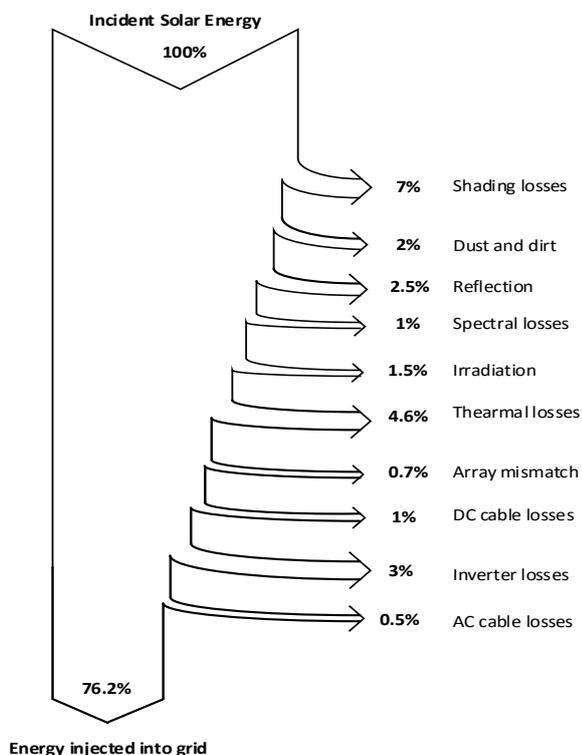
Fig. 1. PV system losses.
