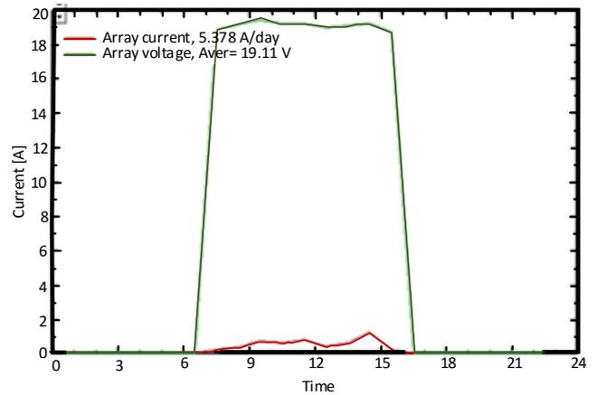
Fig. 7. Current and voltage curve of selected PV module.
