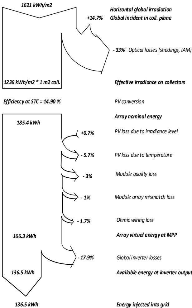
**Fig. 8.** System loss diagram of conductor which has 1.5 mm<sup>2</sup> cross sectional area.
