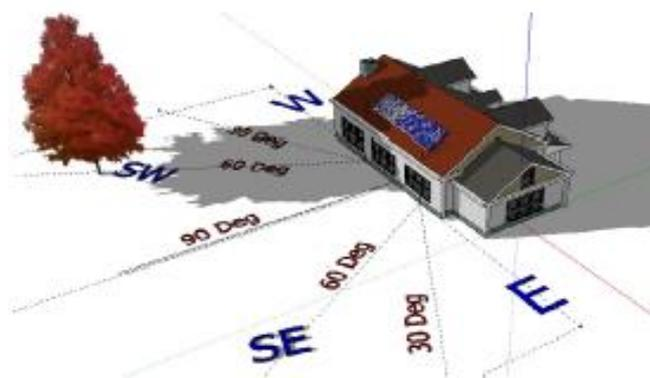
Fig. 2. A solar panel exposed to shading
