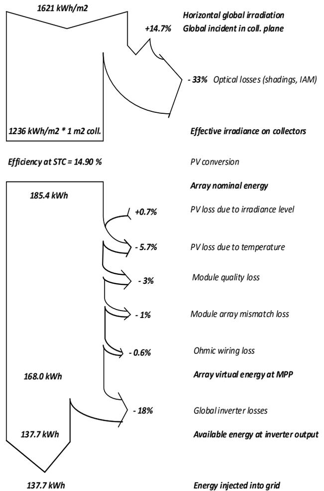
**Fig. 9.** System loss diagram of the conductor which has 4 mm<sup>2</sup> cross-sectional area.
