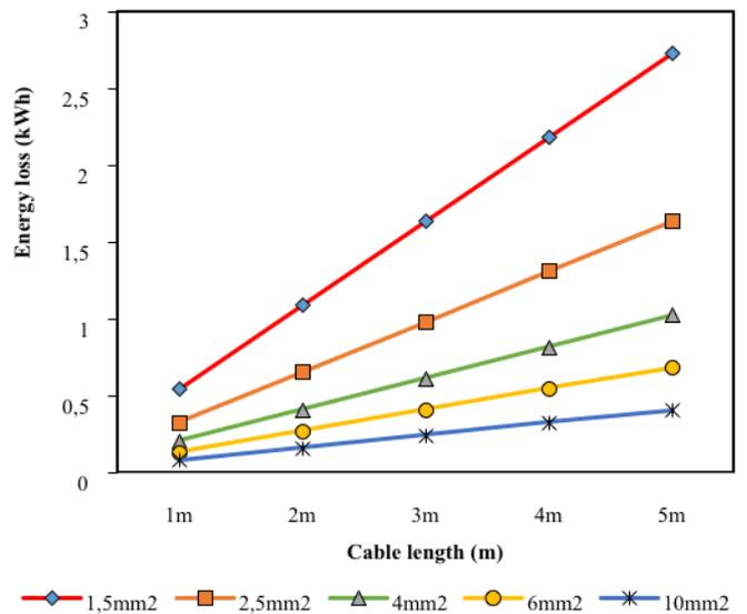
**Fig. 10.** Energy losses for different cable length and cross-sectional area.
