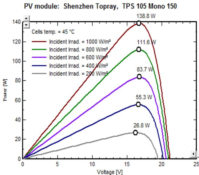
Fig. 6. Power and voltage curve of selected PV module.
