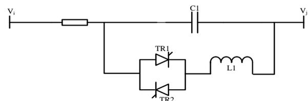
Fig. 2 TCSC connected in a transmission line
