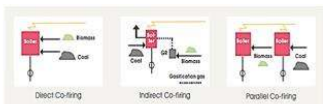
Fig. 3: Different Biomass Co-firing Configurations [15].
