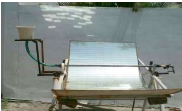
Figure 2 – Fabricated cylindrical parabolic solar collector with glass plate
