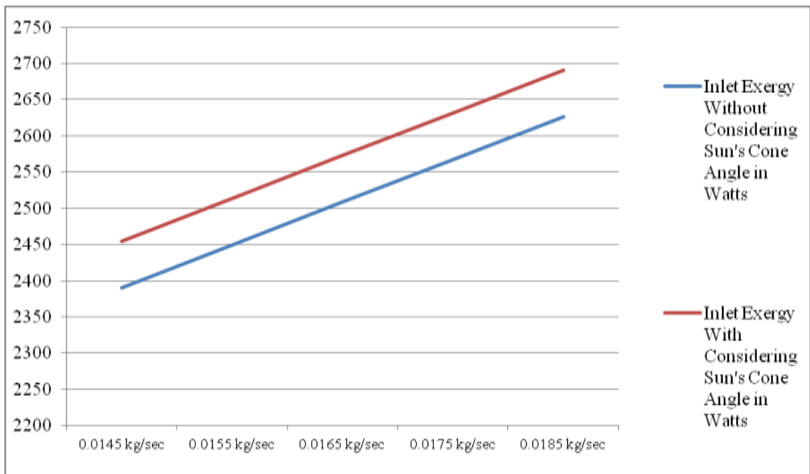
Figure 6 – Inlet exergy curves with different mass flow rates for copper-water arrangement
