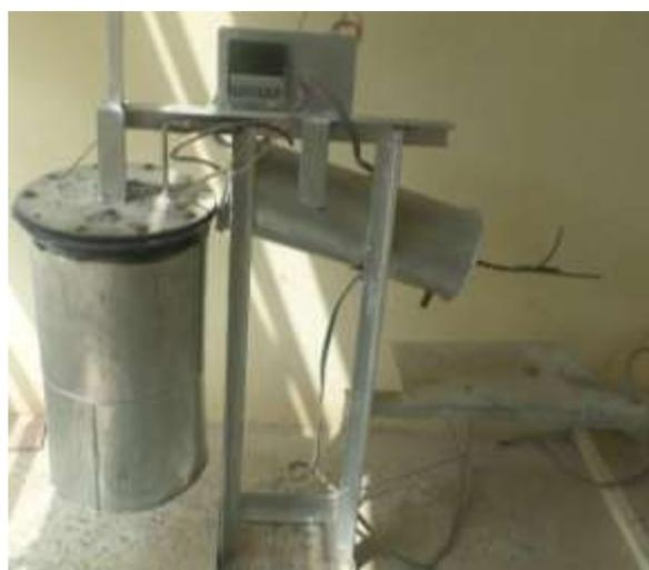
Fig. 5. Pictorial view of the experimental pyrolytic reactor
