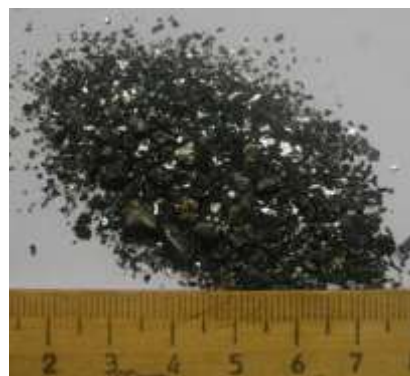
Fig.3. Flakes of the cleaned silicon after treatment with a hydrochloric acid solution.
