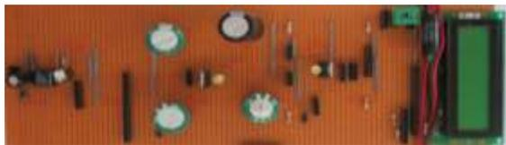
Fig. 5.4: Energy Harvesting Circuit Built on Stripboard
