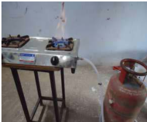
Fig. 6. Burning of bottled Biogas for cooking application
