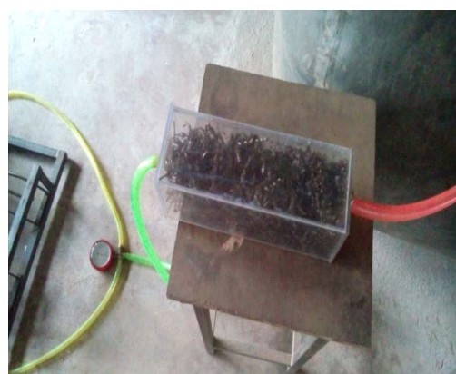
Fig. 3. H 2 S scrubbing mechanism
