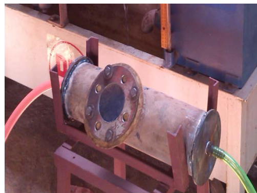
Fig.2. Container with silica gel for removal of water vapour from Biogas
