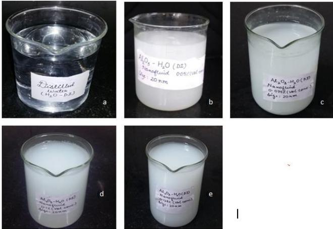
**Figure 3.** Various prepared working fluid: (a) Distilled water, (b) 0.05% vol. conc. Al<sub>2</sub>O<sub>3</sub>-H<sub>2</sub>O (DI), (c) 0.075% vol. conc. Al<sub>2</sub>O<sub>3</sub>-H<sub>2</sub>O (DI), (d) 0.1% vol. conc. Al<sub>2</sub>O<sub>3</sub>-H<sub>2</sub>O (DI), (e) 0.125% vol. conc. Al<sub>2</sub>O<sub>3</sub>-H<sub>2</sub>O
