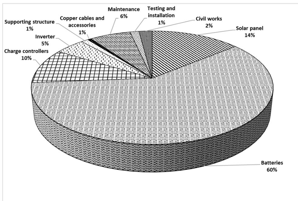
**Fig. 7.** Percentage contribution of the components to the total annualized cost of the system.
