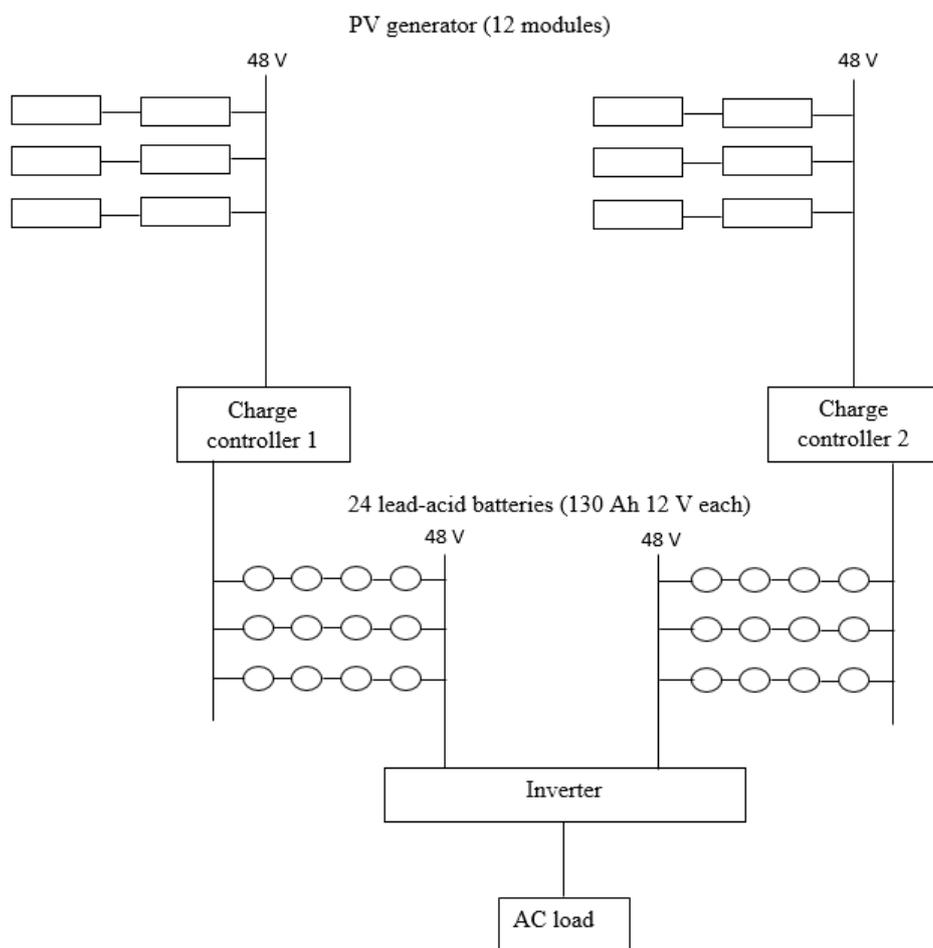
**Fig. 5.** Circuit diagram of the stand-alone PV system.
