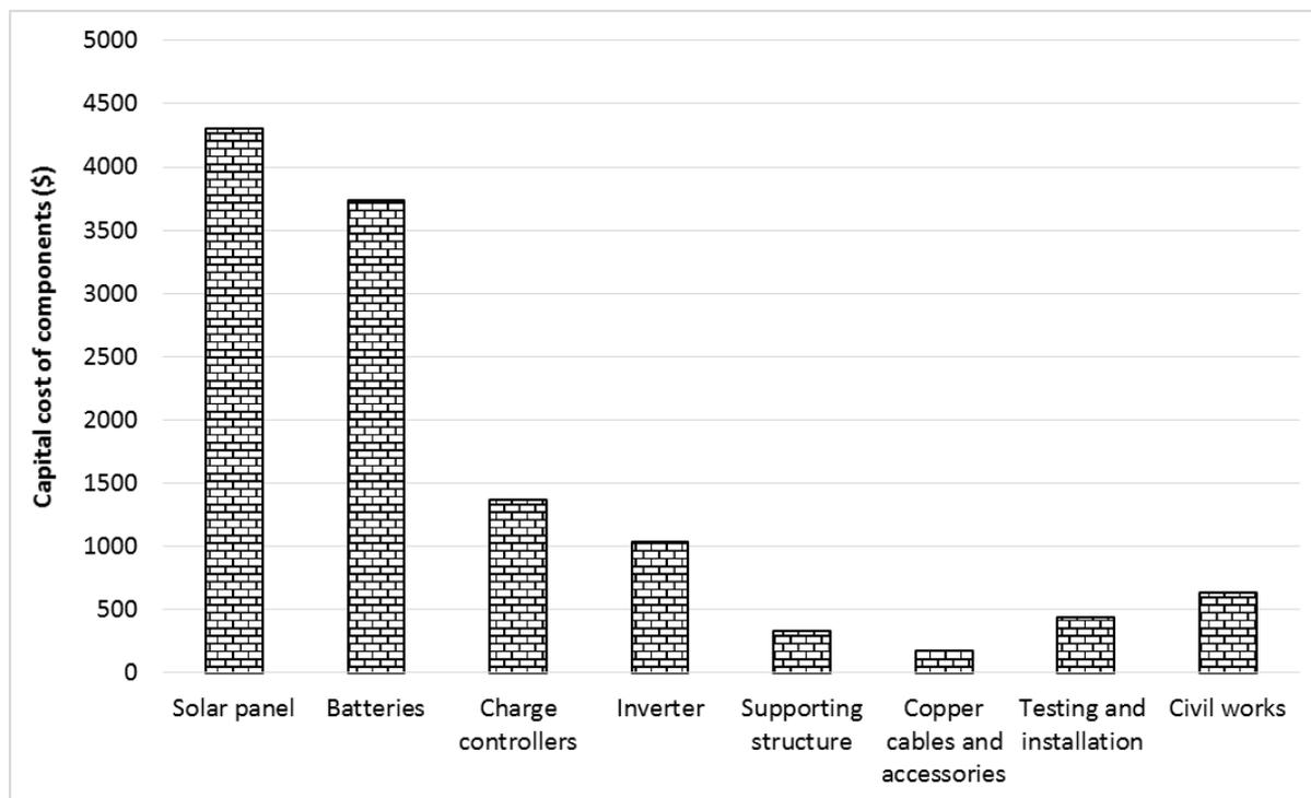
Fig. 6. Capital cost distribution for the solar PV system.
