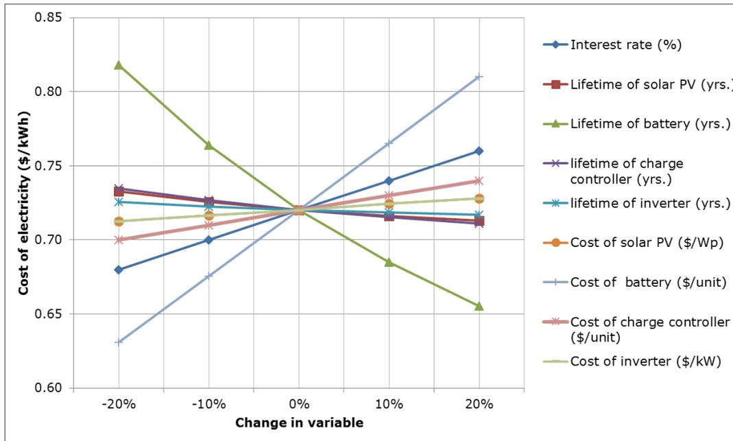
Fig. 8. Sensitivity analysis for the cost of electricity (COE).
