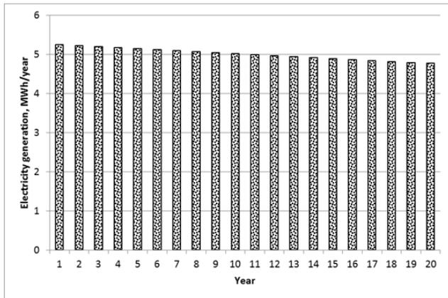
**Fig 4.** Estimated energy production during the life cycle of the PV system.
