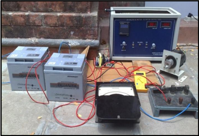
Fig. 12. BLDC motor powered by the batteries with the boost converter
