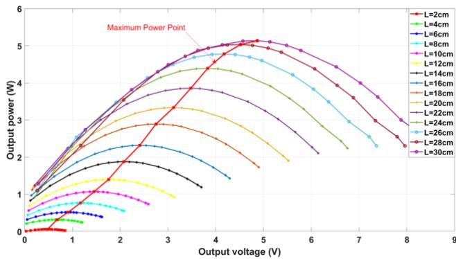
**Fig. 9.** Electric characteristic power-voltage of thermoelectric generator
