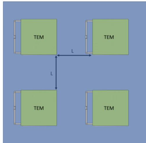
Fig. 4. Positioning structure of TEGs modules
