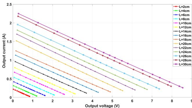
**Fig. 10.** Electric characteristic current-voltage of thermoelectric generator
