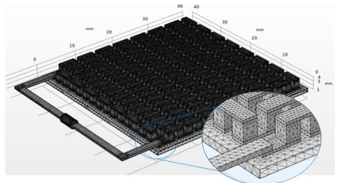
Fig. 5. Geometric structure and TEG grid system
