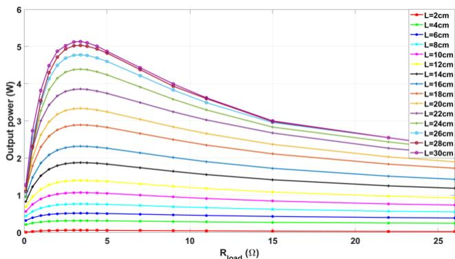
**Fig. 8.** Variation of output power with load resistance
