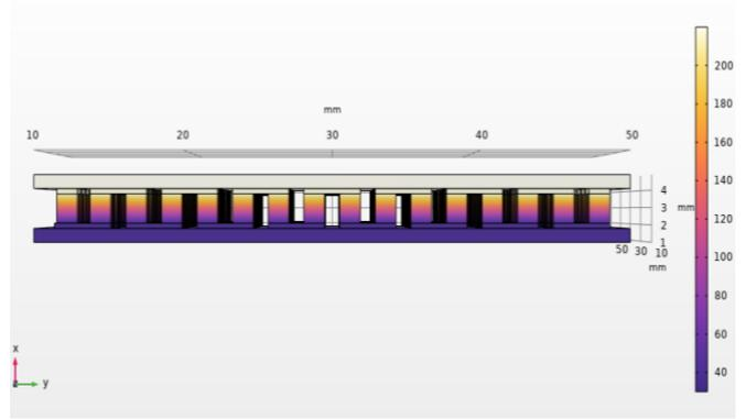
**Fig. 6.** Voltage contour (V) (a) and temperature contour (b) for  $T_H=200^\circ\text{C}$  and  $T_C=30^\circ\text{C}$
