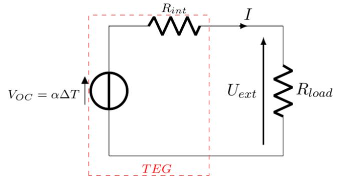
Fig. 1. Electrical equivalent circuit of the TEG
