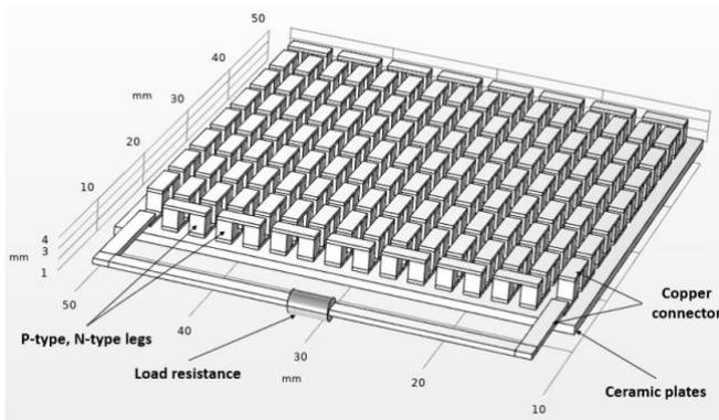
Fig. 2. Three-dimensional geometry of the TEG
