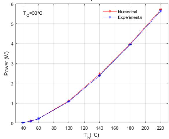
**Fig. 7.** Comparison between numerical and experimental performance curves-open circuit voltage and output power
