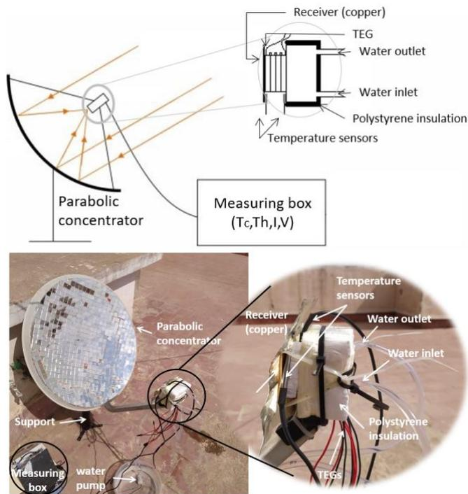
**Fig. 12.** Diagram and realization of a thermoelectric generator with parabolic concentrator and cooling by water circulation
