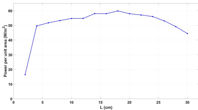
**Fig. 11.** Power per unit area with distance between TEG
