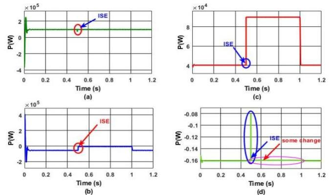
Fig.5 Profile of active powers in PTS without CB (a) Generated power by SPP (b) Grid power (c) Load power (d) Capacitor bank power
