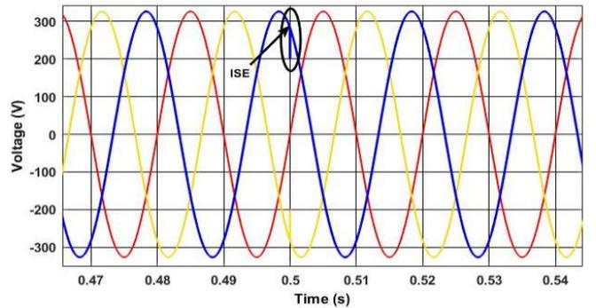
Fig.9 Disturbance detection impact (DDI) in grid voltage signal without CB
