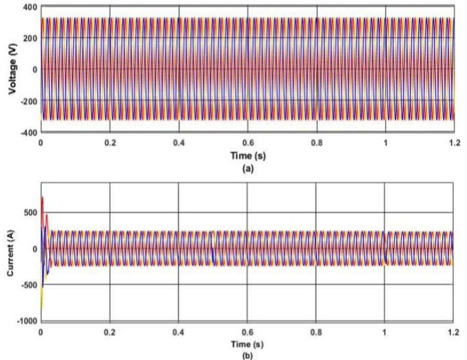
Fig.22 Performance of utility grid parameters with CB (a) Voltage signal profile (b) Current signal profile
