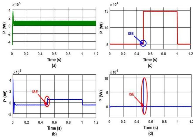
Fig.20 Profile of active powers in PTS without CB (a) Generated power by SPP (b) Grid power (c) Load power (d) Capacitor bank power
