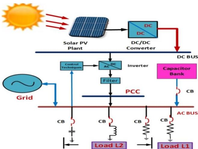
Fig.1 Proposed test system for study of research work
