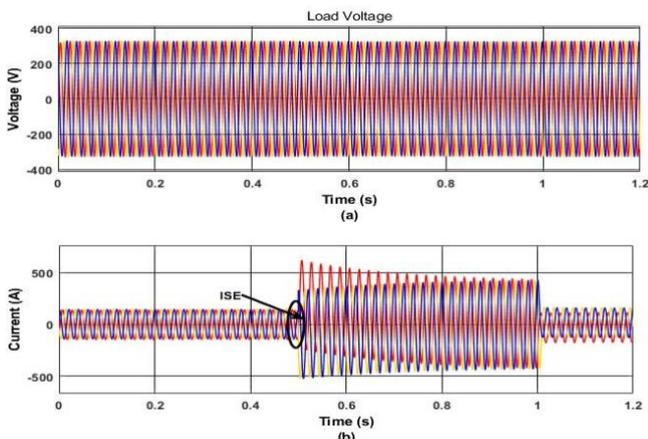
Fig.28 Performance of utility load parameters without CB
