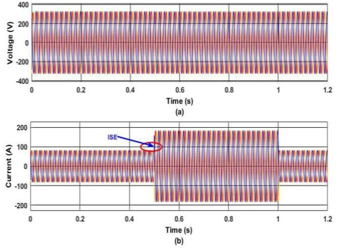
Fig.8 Performance of utility load parameters without CB (a) Voltage signal profile (b) Current signal profile
