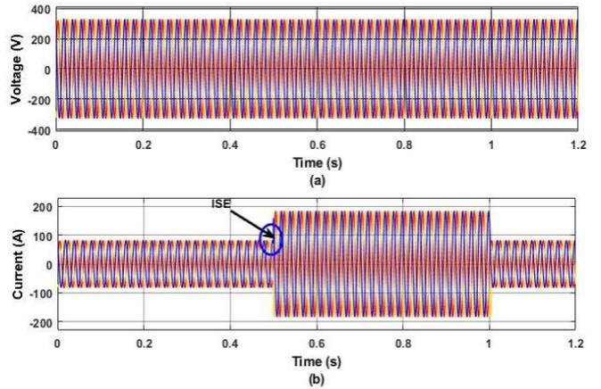
Fig.13 Performance of utility load parameters with CB (a) Voltage signal profile (b) Current signal profile
