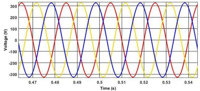
Fig.34 Disturbance detection impact (DDI) in grid voltage signal with CB
