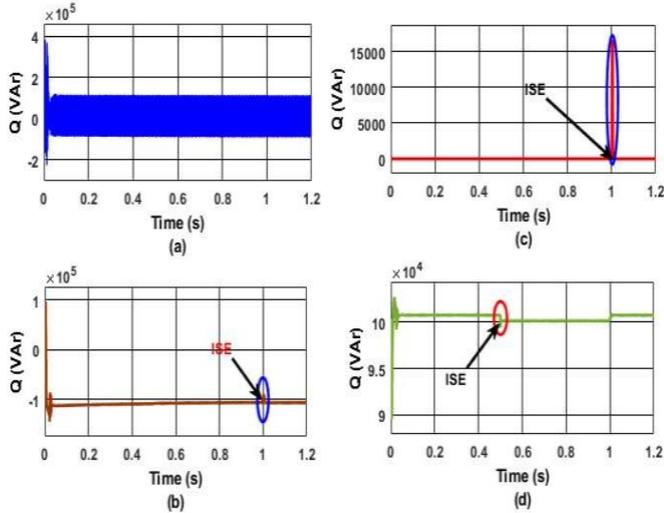
Fig.11 Profile of reactive powers in PTS with CB (a) Solar power (b) Grid power (c) Load power (d) Capacitor bank power
