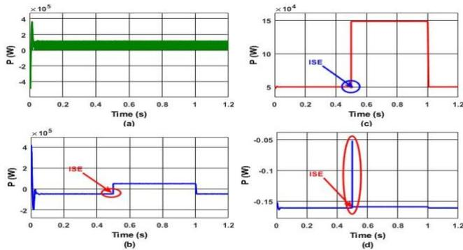
Fig.15 Profile of active powers in PTS without CB (a) Generated power by SPP (b) Grid power (c) Load power (d) Capacitor bank power
