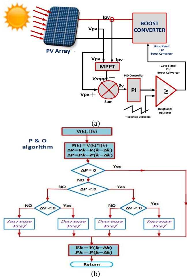
Fig.3 Maximum DC power tracking approach (a) Control structure for boost converter (b) Flow chart for implementation of algorithm for MPPT
