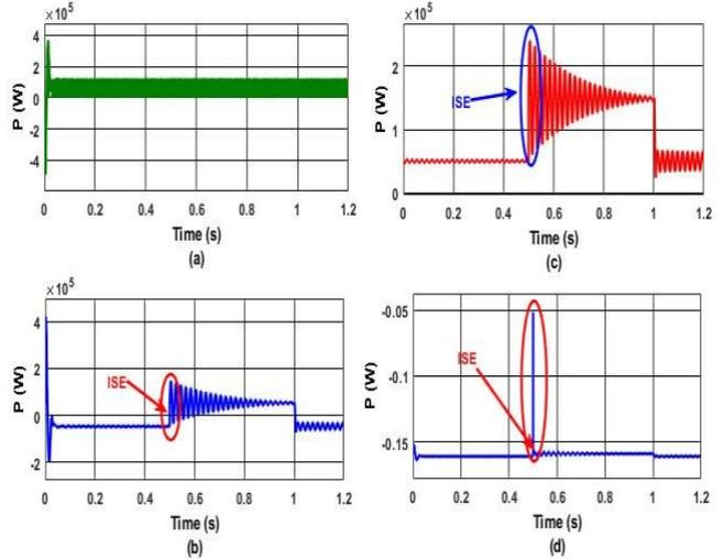
Fig.25 Profile of active powers in PTS without CB (a) Generated power by SPP (b) Grid power (c) Load power (d) Capacitor bank power
