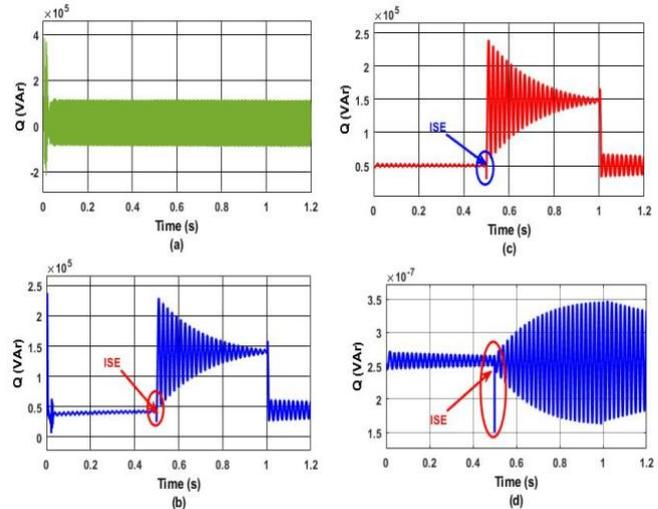
Fig.26 Profile of reactive powers in PTS without CB (a) SPP power (b) Grid power (c) Load power (d) Capacitor bank power
