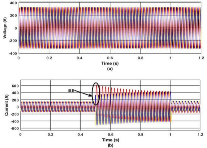
Fig.33 Performance of utility load parameters with CB (a) Voltage signal profile (b) Current signal profile
