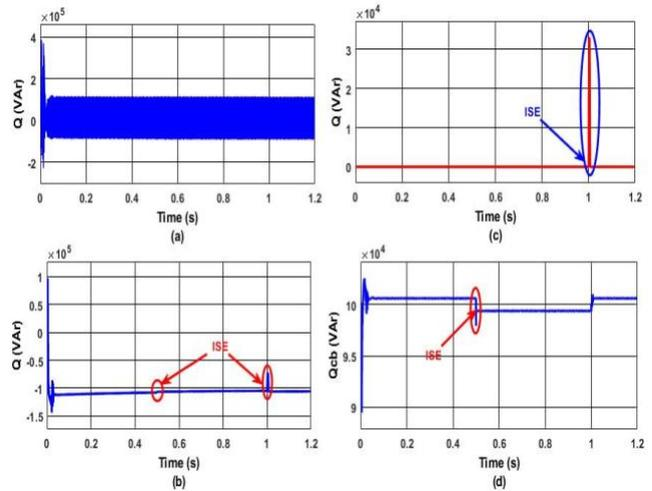
Fig.21 Profile of reactive powers in PTS with CB (a) SPP power (b) Grid power (c) Load power (d) Capacitor bank power
