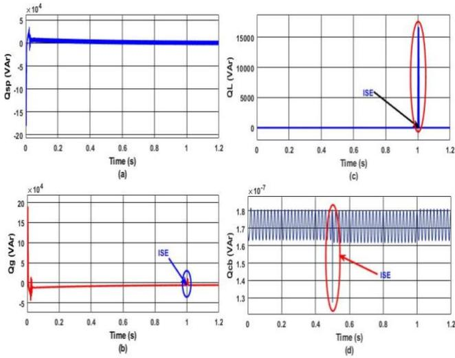
Fig.6 Profile of reactive powers in PTS without CB (a) Generated power by SPP (b) Grid power (c) Load power (d) Capacitor bank power
