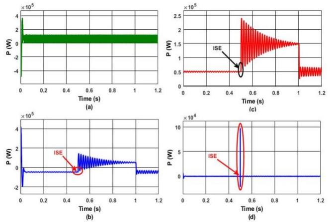
Fig.30 Profile of active powers in PTS with CB (a) Generated power by SPP (b) Grid power (c) Load power (d) Capacitor bank power
