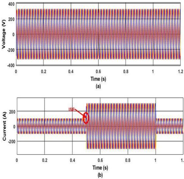
Fig.23 Performance of utility load parameters with CB (a) Voltage signal profile (b) Current signal profile
