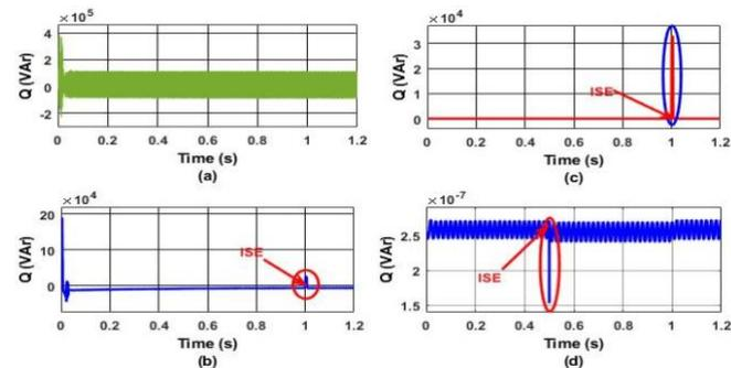
Fig.16 Profile of reactive powers in PTS without CB (a) Generated power by SPP (b) Grid power (c) Load power (d) Capacitor bank power
