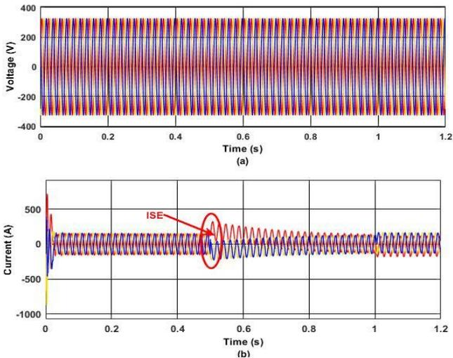
Fig.32 Performance of utility grid parameters with CB (a) Voltage signal profile (b) Current signal profile
