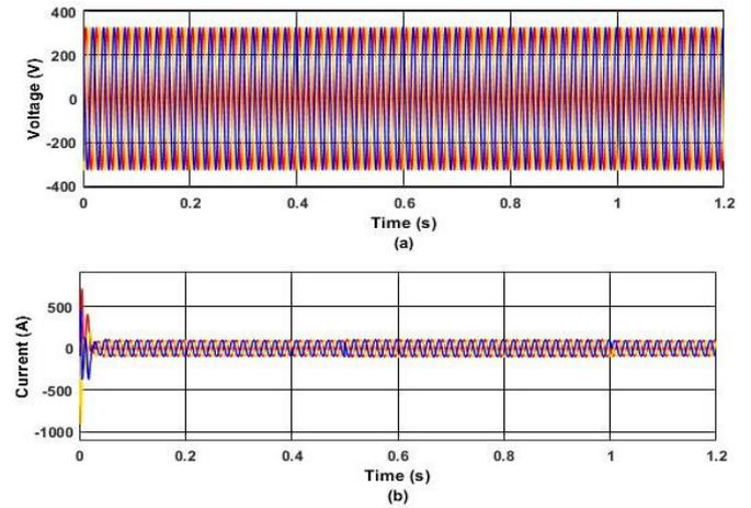
Fig.17 Performance of utility grid parameters without CB (a) Voltage signal profile (b) Current signal profile
