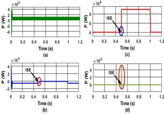
Fig.10 Profile of active powers in PTS with CB (a) Generated power by SPP (b) Grid power (c) Load power (d) Capacitor bank power
