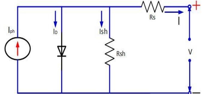
Fig.2 Circuit representation of single solar pv cell for modelling
