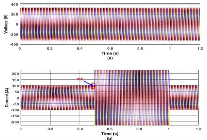
Fig.18 Performance of utility load parameters without CB (a) Voltage signal profile (b) Current signal profile
