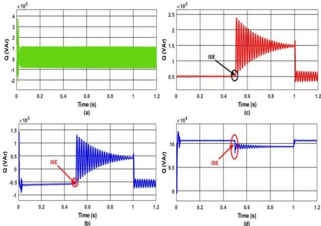
Fig.31 Profile of reactive powers in PTS with CB (a) SPP power (b) Grid power (c) Load power (d) Capacitor bank power
