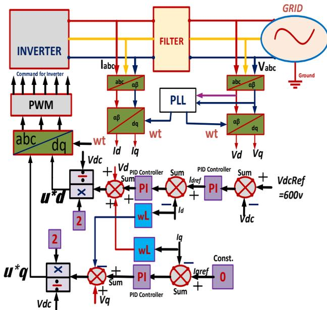
Fig.4 Control structure for inverter voltage control with getting AC maximum power.
