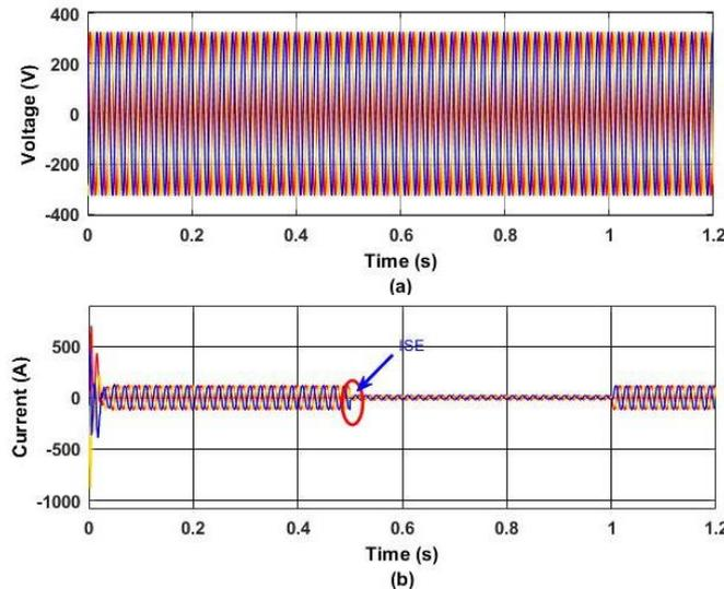
Fig.7 Performance of utility grid parameters without CB (a) Voltage signal profile (b) Current signal profile
