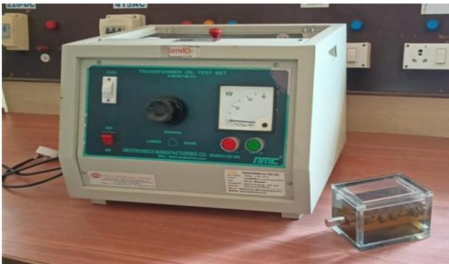
**Fig. 5.** Transformer oil apparatus
