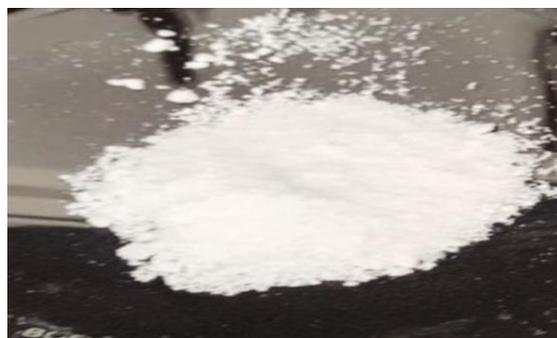
**Fig.2.** TiO<sub>2</sub> Nanopowder
