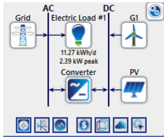
Fig. 4. schematic of the studied hybrid RE system
