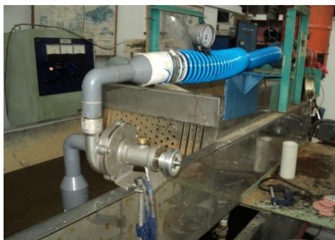
Fig. 5. 1-inch PAT test installation
