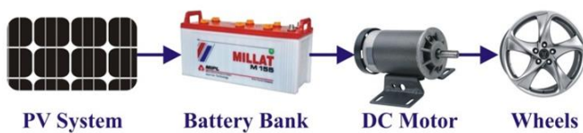
Fig. 1. Basic schematic configuration of solar EVs
