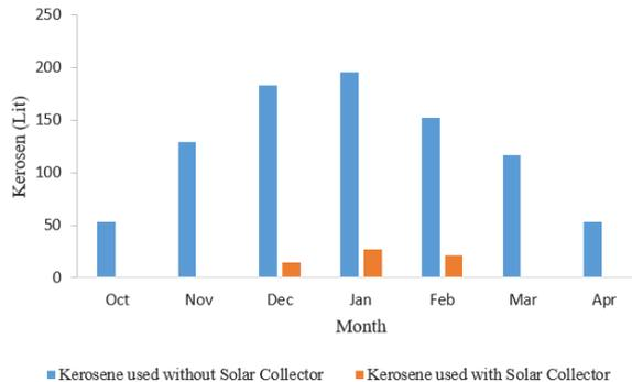
**Fig. 10.** Kerosene used with and without using the solar collector.
