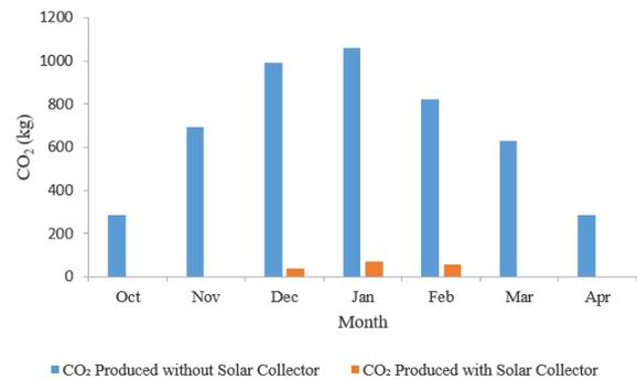
**Fig. 11.** CO<sub>2</sub> emission with and without using the solar collector.
