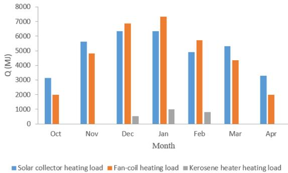
**Fig. 9.** Heat energy required from heaters to recover room heating load.
