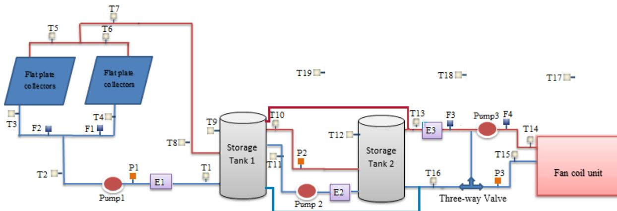
Fig. 2. Solar water heating system layout.
