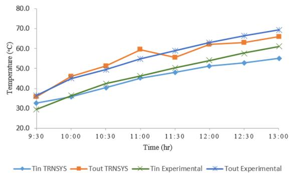
**Fig. 8.** Verification between experimental and simulated solar collector average inlet and outlet water temperature.
