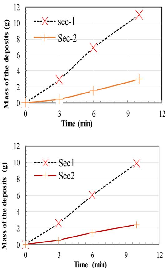
Fig. 4. a) No Load Condition at EGT 120°C- 21.26 kg/h b) Full Load Condition at EGT 180°C, 28 kg/h
