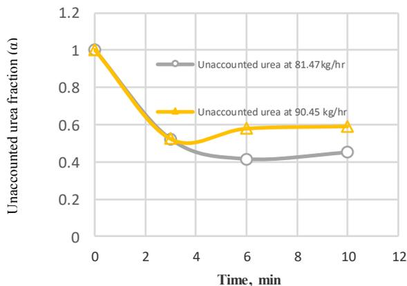
**Fig.9.** Unaccounted urea fraction vs. time for 407 engines run at no load and full load conditions with biodiesel.
