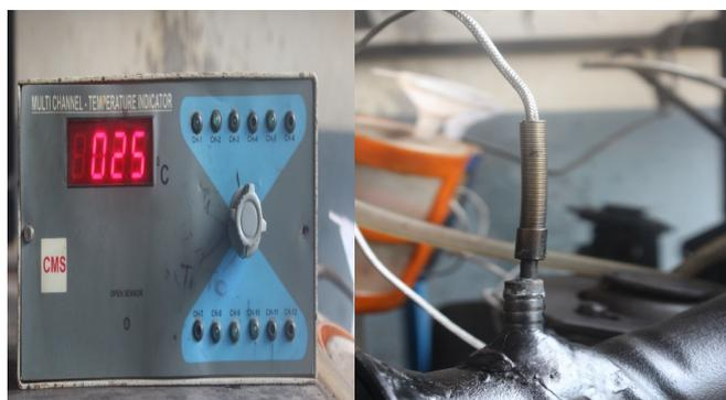
**Fig. 2** a) Temperature Display b) Thermocouple
