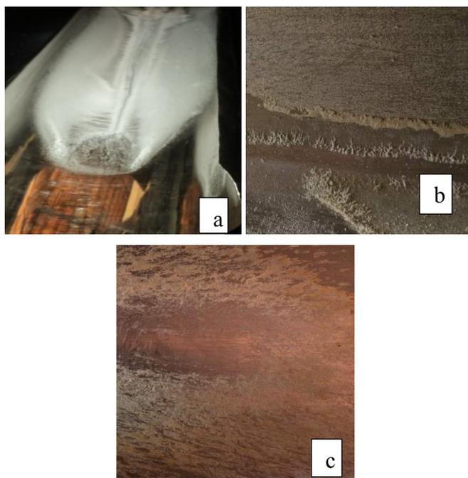
**Fig.7.** Physical nature of deposits a) pure air [21] b) Diesel c) Biodiesel.
