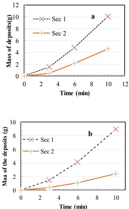
**Fig. 5.** Mass of deposits vs Time, when run with diesel (a) at EGT- 90°C, 81.47 kg/h (b) at EGT- 120°C, 90.45kg/h.
