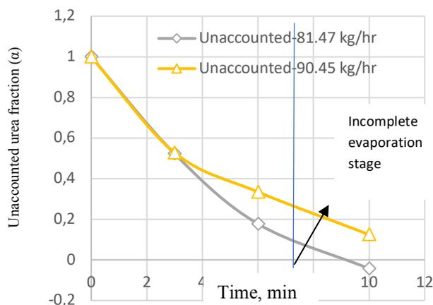
**Fig.8.** Unaccounted urea fraction vs. time for 407 engines at no load and full load conditions running with diesel.
