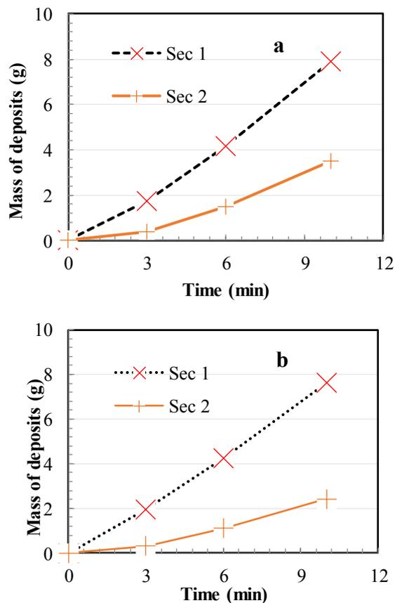
**Fig.6.** Mass of deposits vs Time, when run with biodiesel (a) at EGT- 90°C, 81.47 kg/h (b) at EGT- 120°C, 90.45kg/h.
