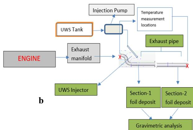
**Fig.1.** a) Experimental Setup b) Detailed diagram UWS injection and Deposit collection.
