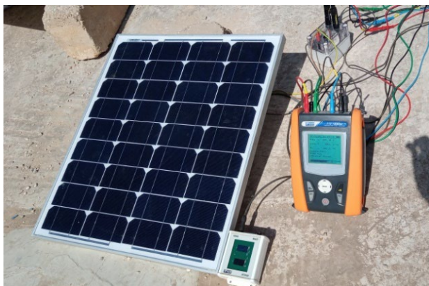
Fig. 15. I-V measurements of the PV module 50W with an I-V 400 W
