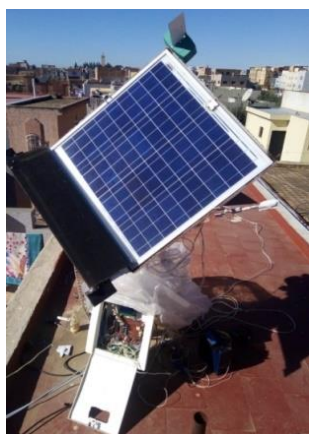
Fig. 28. The equatorial bi-axial solar tracker used in the experiment.
