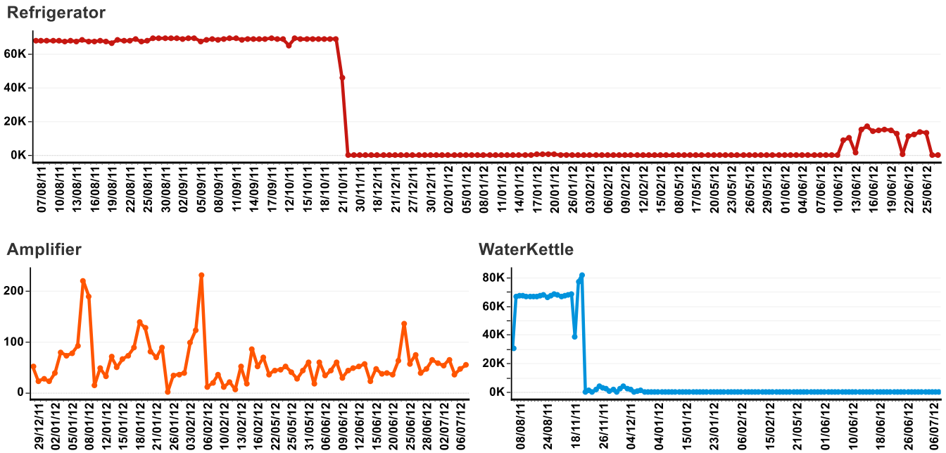
Fig. 3. Quantification of identified redundant data anomalies in different appliances (x-axis represents the date and y-axis represents the count of redundancies corresponding to that date in all the subplots).
