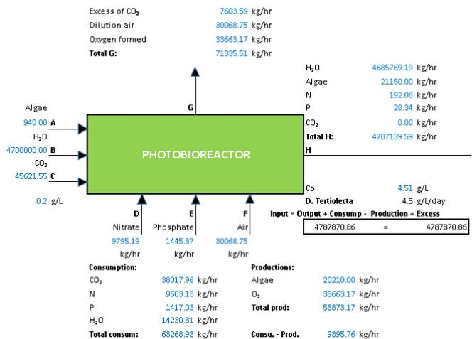
**Fig. 9.** Mass balance for the Vertical tubular serpentine type photobioreactor (Own elaboration)
