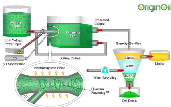
Fig. 5. OriginOil Single-Step Extraction™ method
