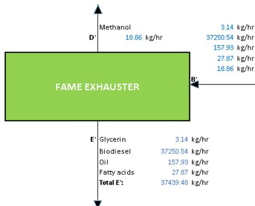
**Fig. 14.** Mass balance in the separation phase of biodiesel and glycerin (Own elaboration)
