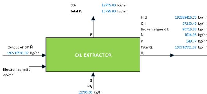
**Fig. 11.** Mass balance in the biodiesel extraction phase (Own elaboration)
