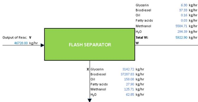
**Fig. 13.** Mass balance in the separation phase of biodiesel and methanol (Own elaboration)
