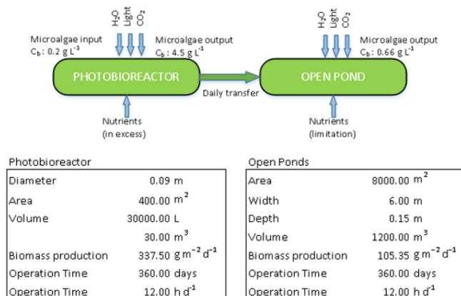
Fig. 7. Block diagram of the mixed or hybrid culture phase (Own elaboration)
