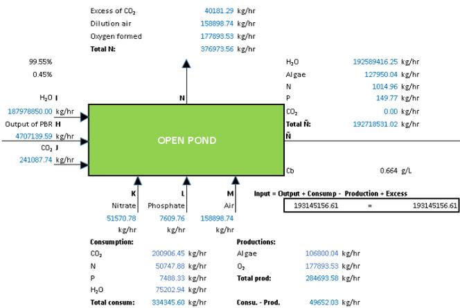
**Fig. 10.** Mass balance for the open raceway pond (Own elaboration)
