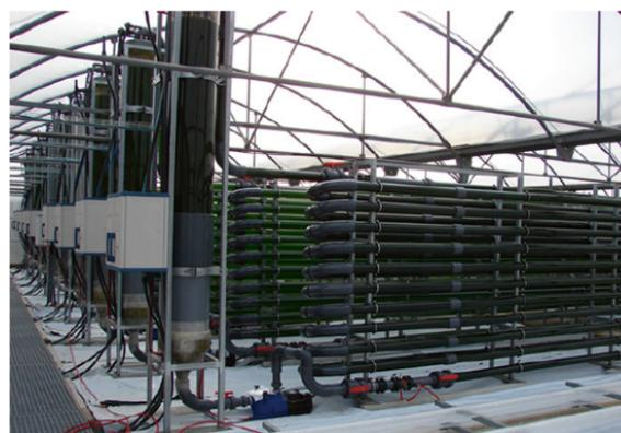
Fig. 8. Vertical tubular serpentine photobioreactor of Almería (Spain)
