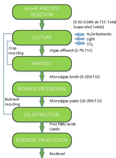
**Fig. 4.** Overview of biodiesel production processes from microalgae (Own elaboration)
