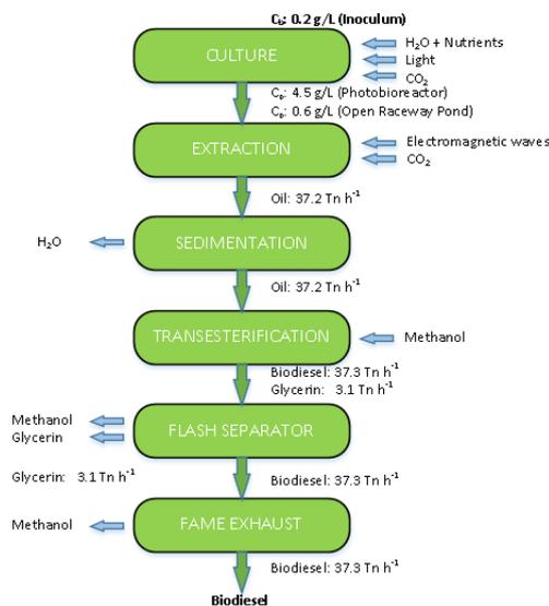
**Fig. 6.** Overview of the production processes of biodiesel from microalgae considered in this research (Own elaboration)
