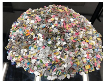
Fig. 1. The feedstocks from aseptic packaging wastes after cutting.
