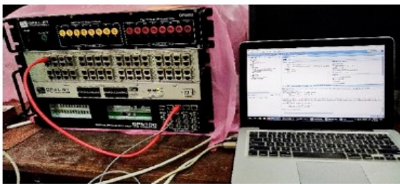
Fig.11 (a). OPAL-RT simulator setup
