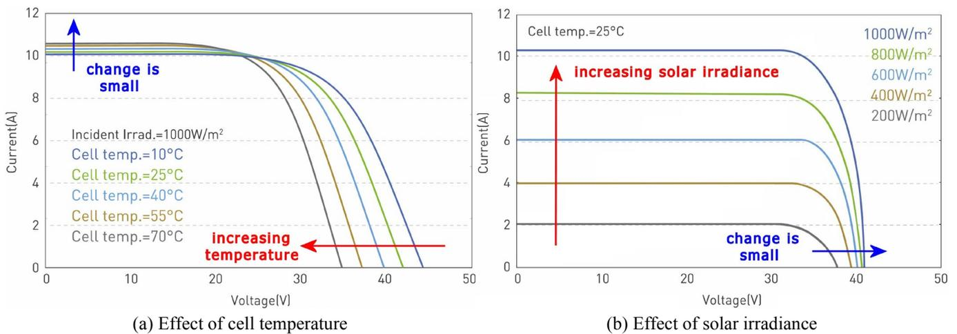
**Fig. 4.** The effect of increasing cell temperature and solar irradiance on I-V curves.
