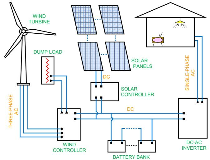
**Fig. 2.** Schematic view of the considered wind-solar-battery system.
