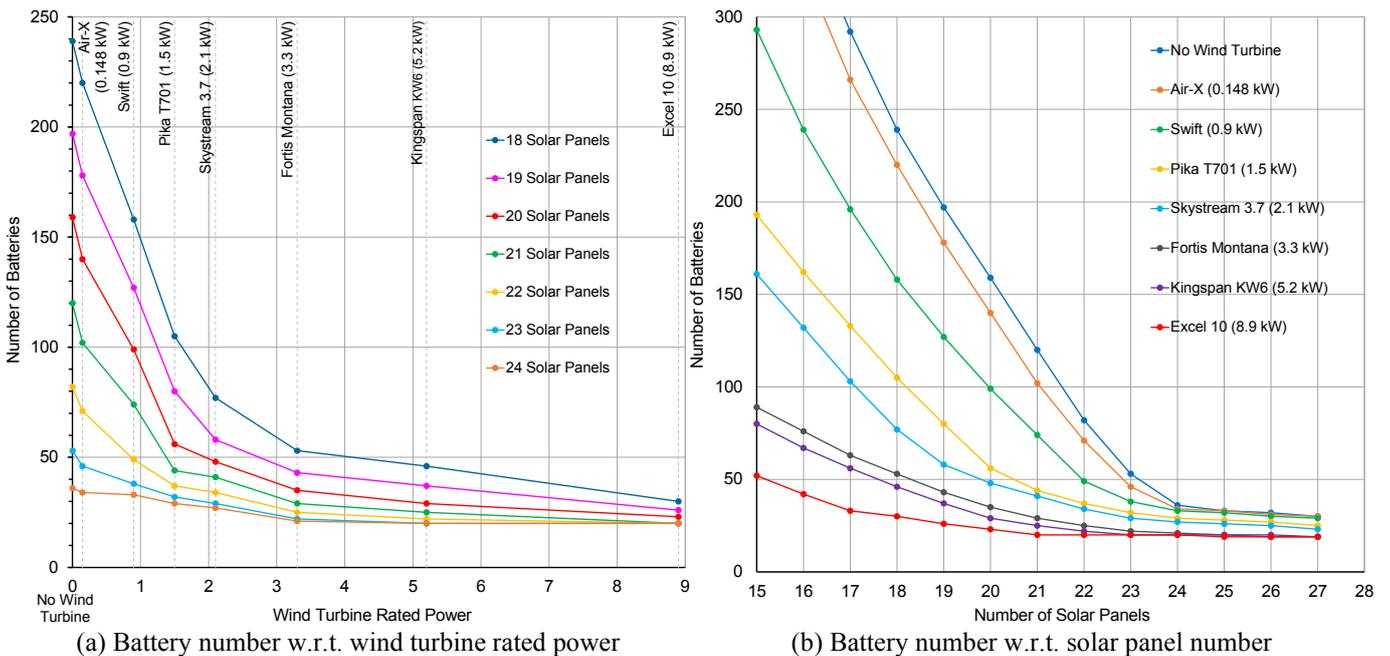
Fig. 9. Change in minimum number of battery in the system.
