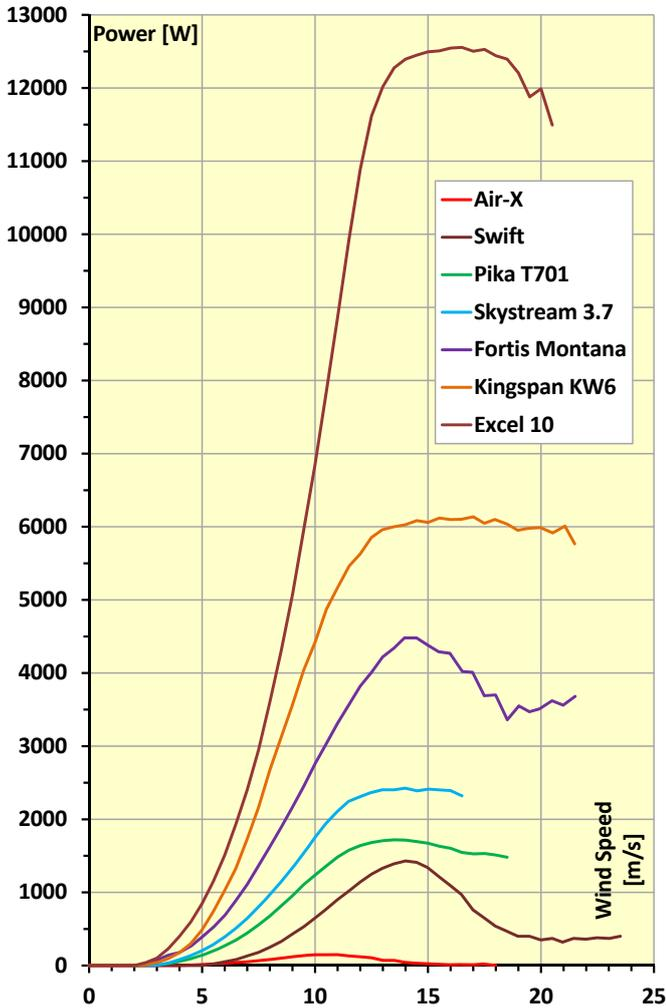
Fig. 3. Wind turbine's power curves.
