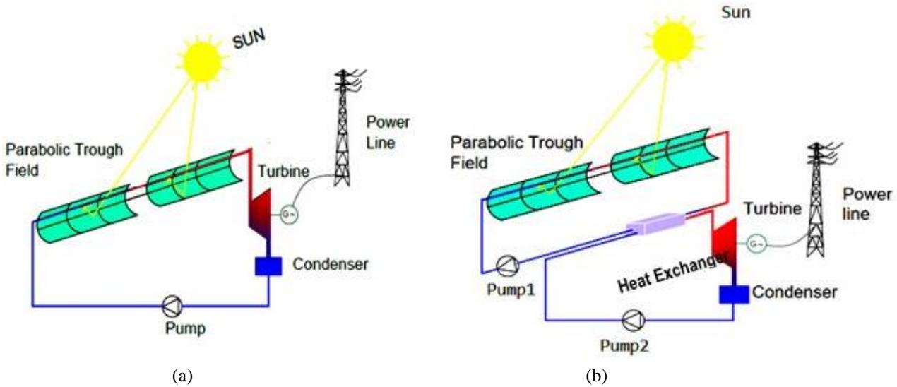
**Fig 1.** Direct (a) and (b) indirect steam generation systems
