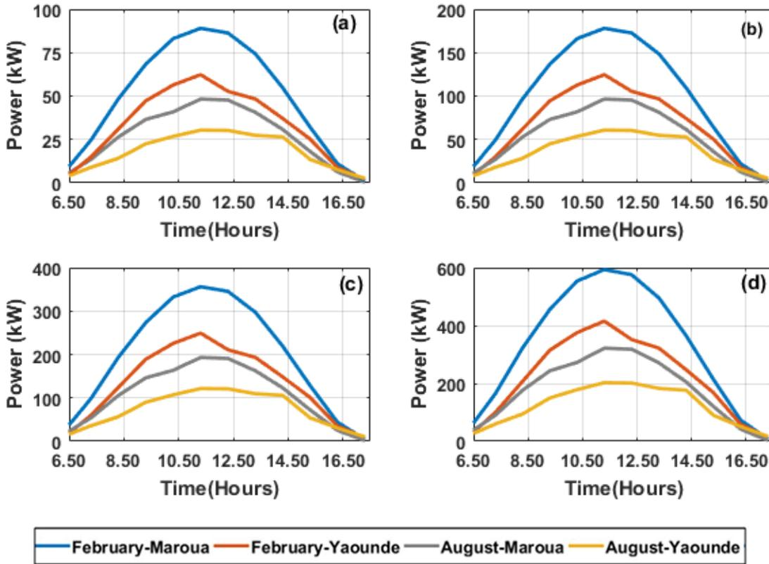
**Fig. 11.** Output power of steam for (a) one, (b) two, (c) four and (d) eight PTCs mounted in séries.
