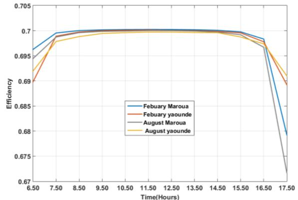
**Fig. 9.** Thermal conversion efficiency for an association of 8 collectors
