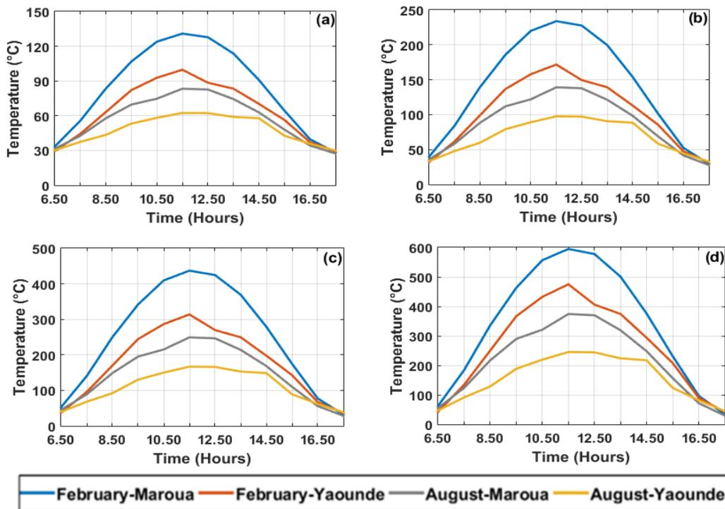
Fig. 7. Water outlet temperature for (a) one, (b) two, (c) four and (d) eight PTCs mounted in series.
