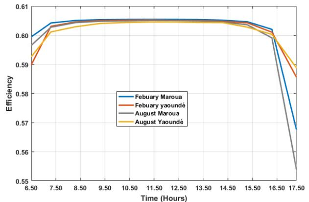
**Fig. 12.** Thermal efficiency for an association of four concentrators.
