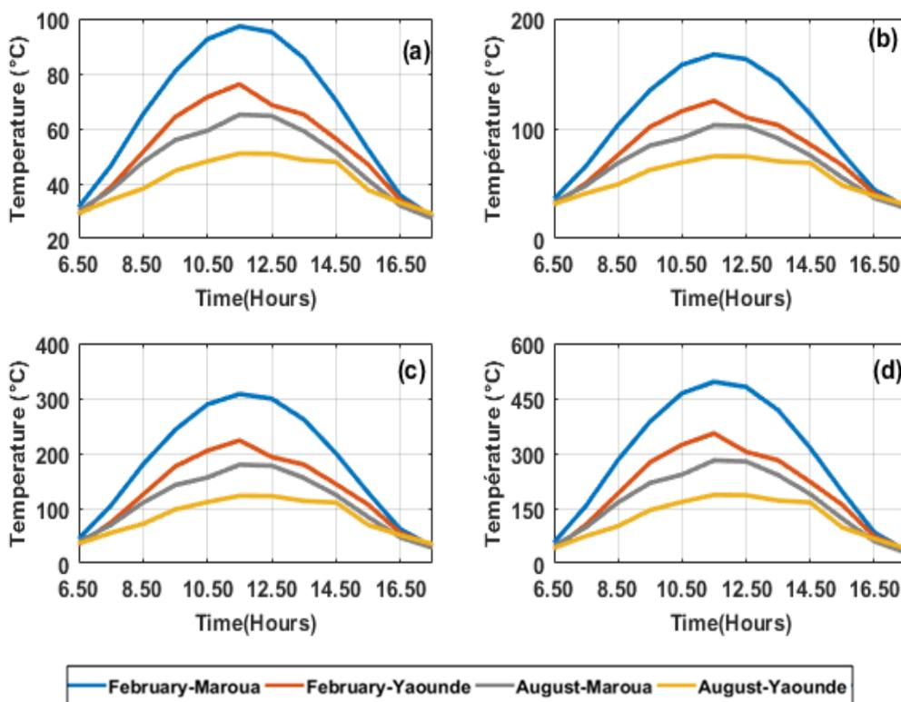
Fig. 10. Water outlet temperature for (a) one, (b) two, (c) four and (d) eight PTCs mounted in series.
