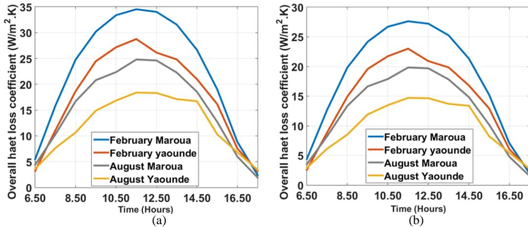
Fig. 6. Profile of the overall heat loss coefficient (a) in direct generation and (b) in indirect generation modes.
