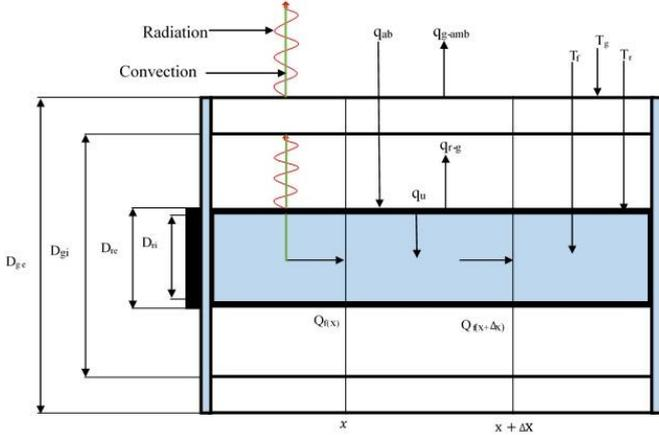
**Fig 3.** Longitudinal section of the absorber tube and heat transfer processes.
