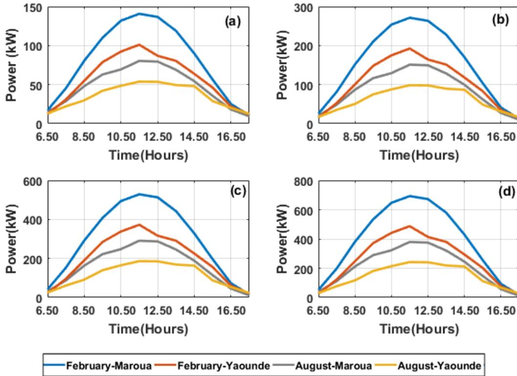
**Fig. 8.** Output power of steam for (a) one, (b) two, (c) four and (d) eight PTCs mounted in Série.
