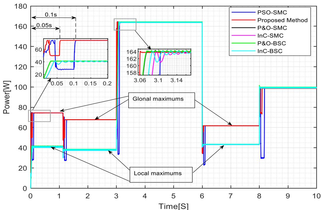
Fig. 9. Comparison of MPPT and GMPPT techniques.
