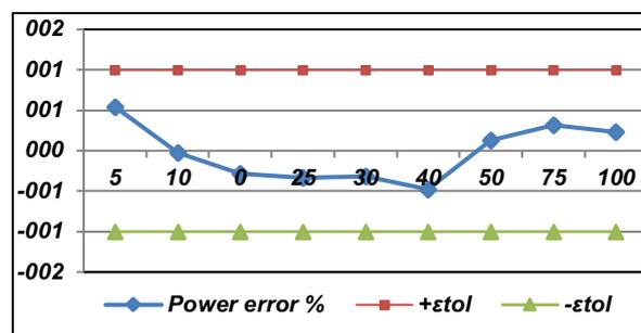
Fig. 12. Power percent relative errors obtained for all power ratios required for the EN 50530 efficiency test conditions.
