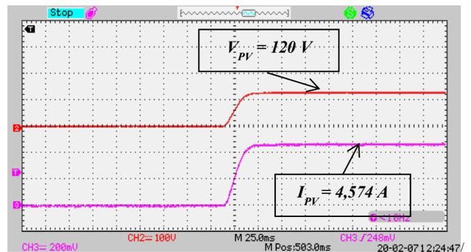
Fig. 9. PVE voltage and current outputs for 50% of  $P_{DC,r}$  under  $T^{\circ}=25\text{ }^{\circ}\text{C}$  and  $G=500\text{ W/m}^2$ .
