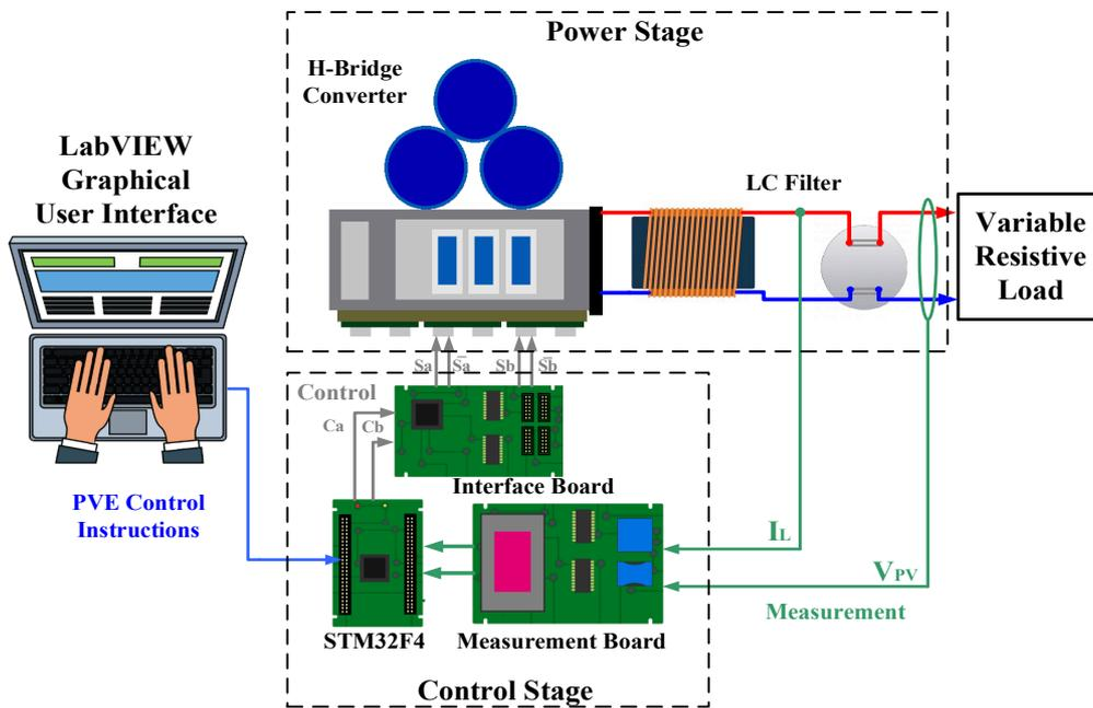
**Fig. 2.** Proposed PVE-based platform and the communication between its components
