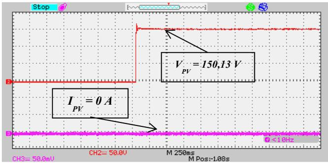
Fig. 7. PVE outputs in Open-circuit operating conditions under  $T=25\text{ }^{\circ}\text{C}$  and  $G=100\text{ W/m}^2$ .
