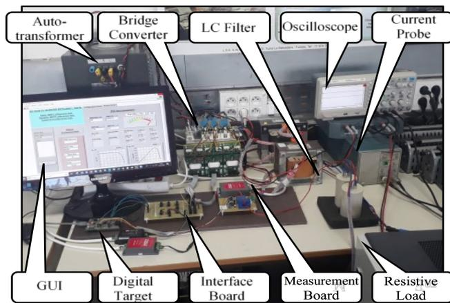
Fig.5. Experimental PVE setup to evaluate the EN 50530 static MPPT efficiency
