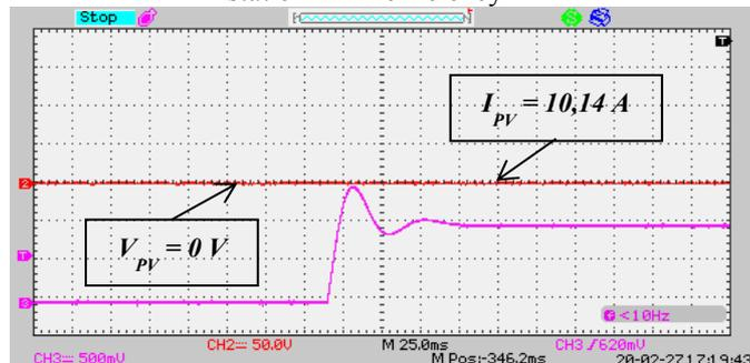
Fig 6. PVE outputs in Short-circuit operating conditions under  $T=25$  °C and  $G=100$  W/m<sup>2</sup>.
