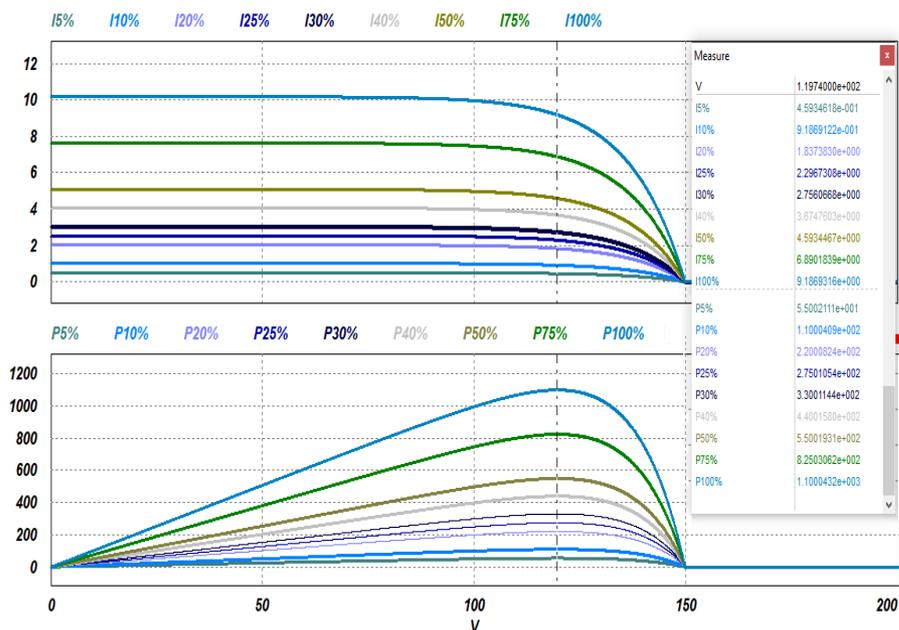
Fig.4. I-V and P-V simulated characteristics for the ENFINITY 100 TL PVI under the EN 50530 standard conditions.
