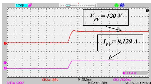
Fig. 10. PVE voltage and current outputs for 100% of  $P_{DC,r}$  under  $T^{\circ}=25^{\circ}\text{C}$  and  $G=1000\text{ W/m}^2$ .
