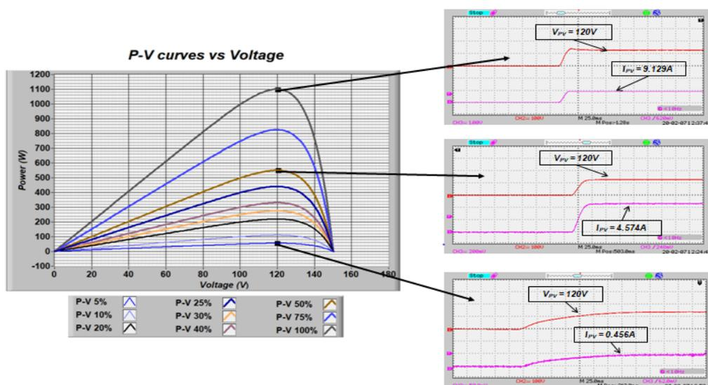
Fig. 11. Experimental emulated P-V characteristics.
