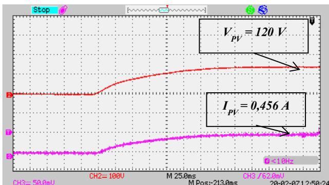
Fig.8. PVE voltage and current outputs for 5% of  $P_{DC,r}$
