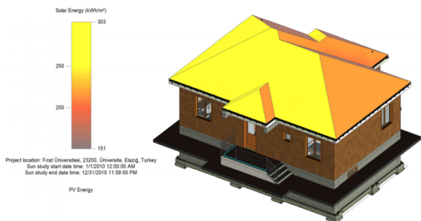
Fig. 1. Analysis of solar radiation falling on the specified house by BIM tool.
