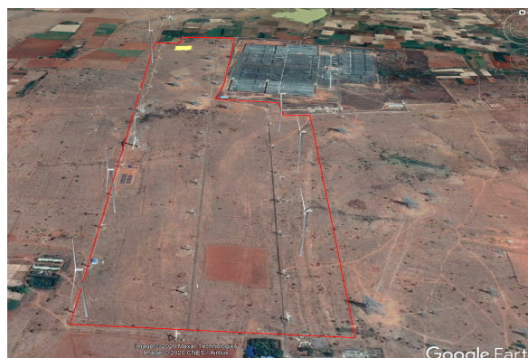
Fig. 9. Layout of substitution of old 200 kW wind turbines with higher capacity wind turbine 3000 kW (higher hub height and longer blades) (Google map)
