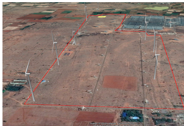
Fig. 8. Layout of substitution of old 200 kW wind turbines with higher capacity wind turbine 2700 kW (higher hub height and longer blades) - (Google map)
