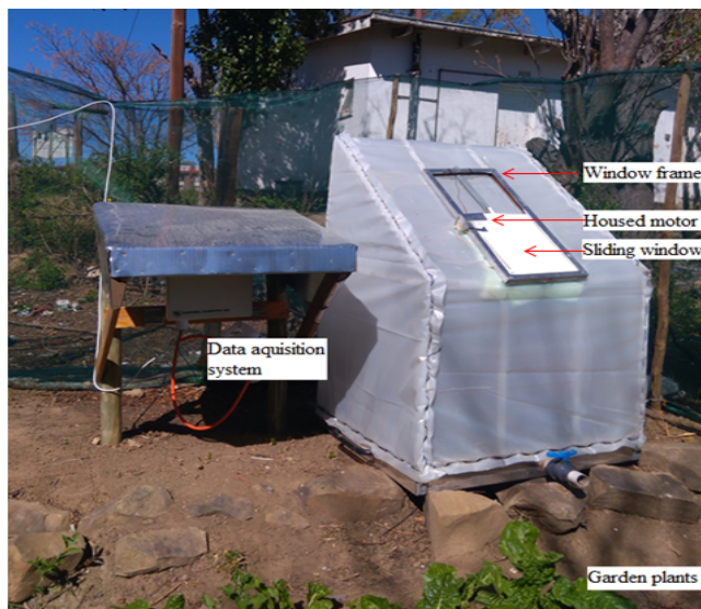
Fig. 3. Greenhouse regulated temperature biogas digester.
