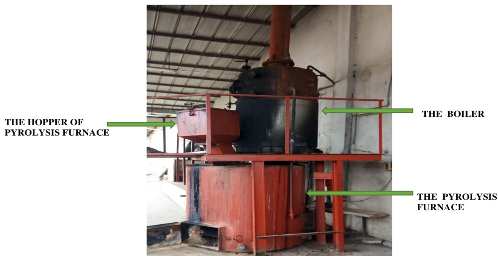
Figure 2. Example of equipment used for the thermochemical treatment of cashew nut shells (Valorization of shells into pyrolysis gas for feeding a boiler)
